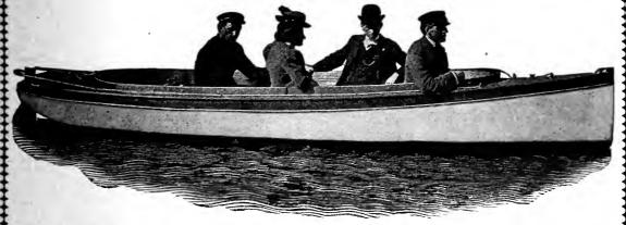
20th Century Electro-Vapor Launch, as shown above, is an ideal gentleman's outfit; 16ft. long, will seat comfortably eight persons and speed 6 miles per hour. Elegantly finished in Solid Oak and Walnut with polished brass trimmings. Steel watertight bulkheads, all screw fastened. Safe, seaworthy, reliable, free from complications and care, over 700 in actual service. Just the outfit for a summer home. Guaranteed for one year or money refunded.
