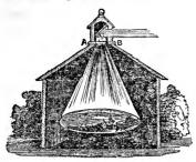
taining from one to eight persons. A B is a sliding piece, having a sloping mirror, C, and a double convex lens, which may, with the mirror C, be slid up or down, so as to accommodate the lens to near or distant objects. When the rays proceeding from an object without fall upon the mirror, they are reflected upon the lens F, and brought to fall on the bottom of the box, or upon a table placed horizon-
