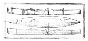
Sections, Lines, Deck and Sheer Plans of a Decked Racing Canor
