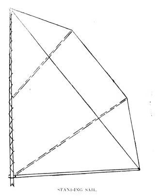
The triangular sail is a leg of mutton with only two spars, boom and mast. The five-sided sail has mast, boom and two battens. Both sails have only one rope—the sheet.
