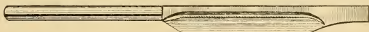
Pattern Blocked Out for Regular Cross-Firing Shoe, Swedged Outside, Half Round Inside.
