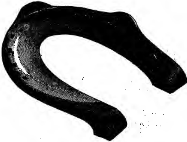
FIG. 498.—Shoe too Wide and Long. Bearing-surface too Concave.
