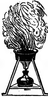
FIG. 1147.—Apparatus for Liberating Sulphuric Acid Gas.
