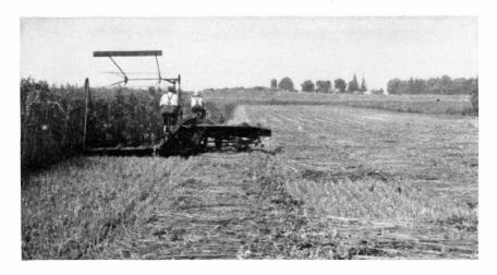
binds the hemp into bundles, is also available, although difficulty in handling the very tall hemp may be experienced. This latter type of machine can be used for short hemp in areas, such as Kentucky, where hemp must be shocked within a few days after harvest to avoid sunburn.
