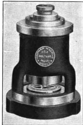
FIG. 5. — Cylindrical sub press with dies for a watch wheel
