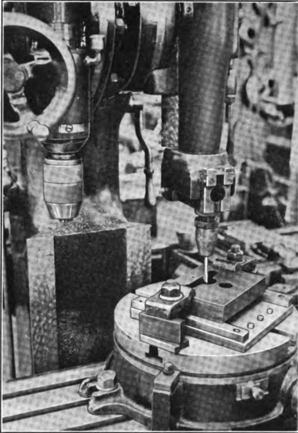
FIG. 562. — Slotting out a die opening
