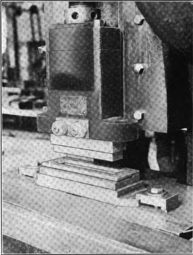
FIG. 389. — Blanking dies in operation
