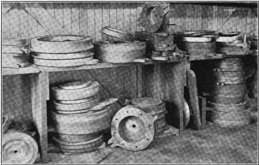
FIG. 280. — Large cast iron drawing and forming dies
