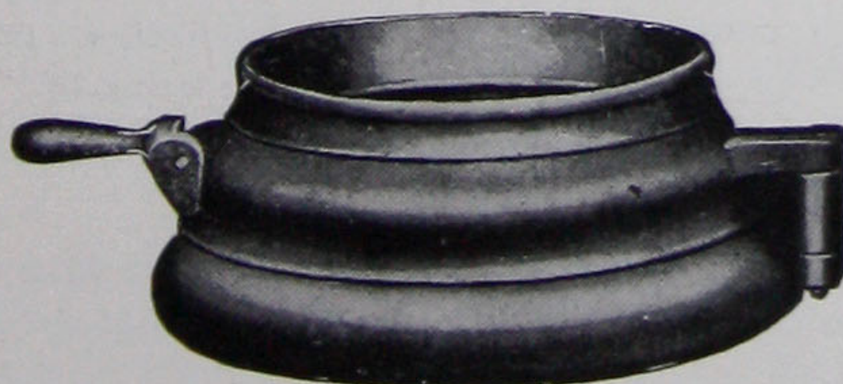
Column Base Mold
