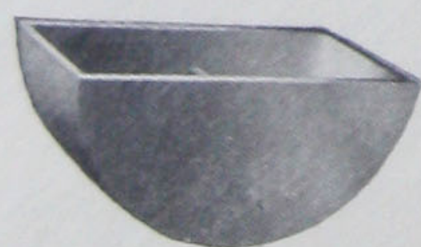
Chimney Stove Pipe Mold
