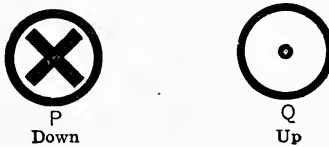
FIG. 2.—Direction of an electric current.
