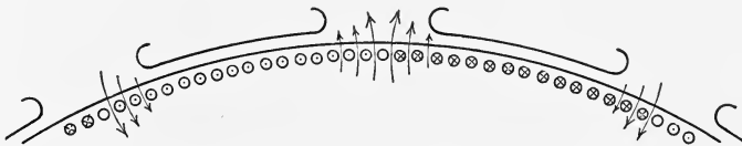
FIG. 74.—Field due to the armature m.m.f.
