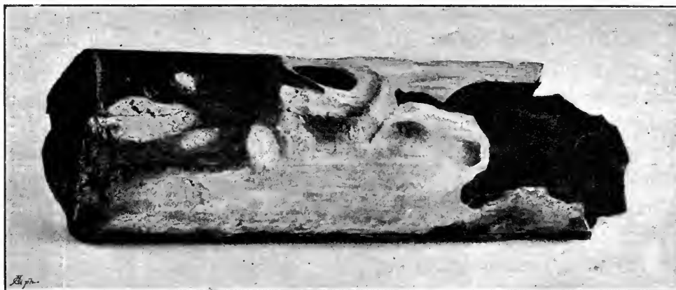
FIG. 37. PIPE CORRODED BY ELECTROLYTIC ACTION OF THE RETURN CURRENT.
