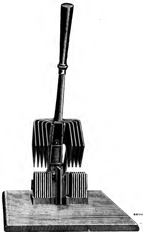
FIG. 290. “AJAX” QUICK-BREAK SWITCH.
