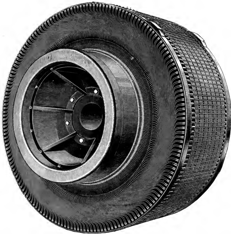
FIG. 256. ARMATURE OF GENERAL ELECTRIC COMPANY'S RAILWAY GENERATOR.
