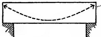
Fig. 50. Anchored End Bar Construction.
