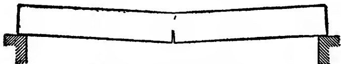
Fig. 46. Plain Concrete Beam.
