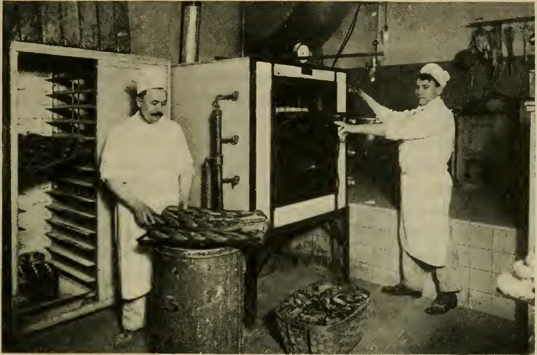
Electric restaurant oven for baking rolls.
