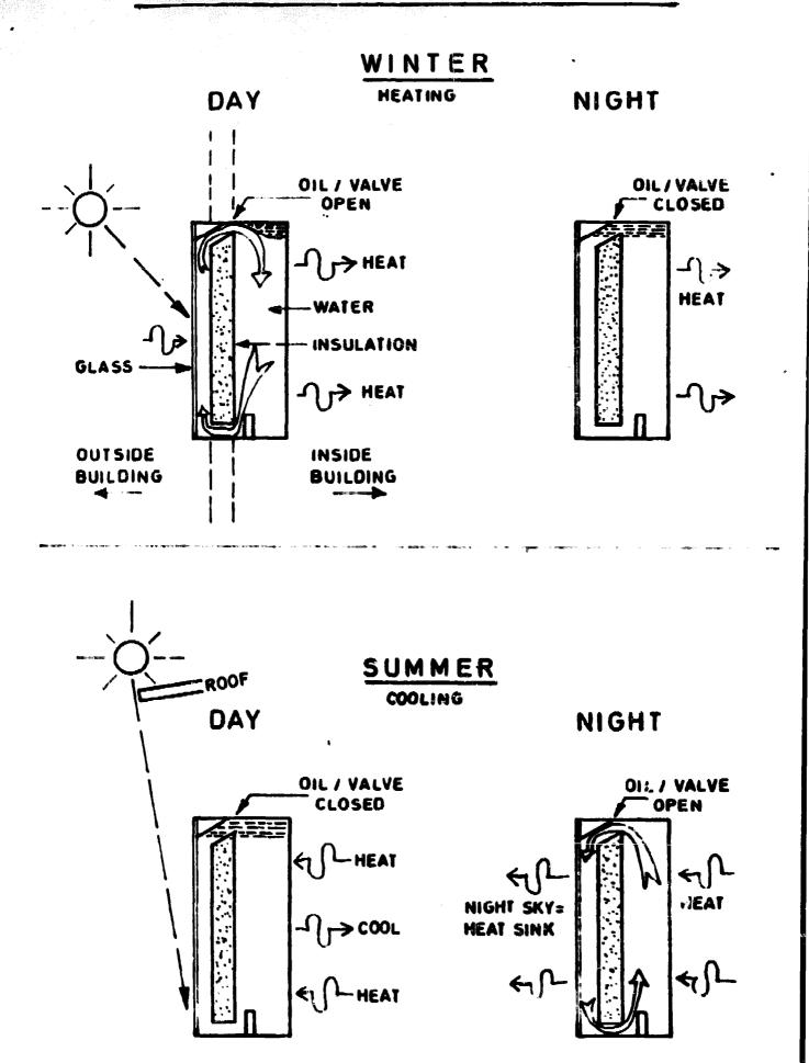
place during the day but is allowed during the night. Then the warmer water convects from the main compartment over the insulation, radiates the heat to the night environment and returns cooled below the insulation to the main compartment. The cooled water then acts as a heat sink for the building during the day.
