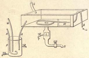
FIG. 7.—SEPARATOR. A, Compressed Air Pipes; G, Nitro-glycerine enters from Nitrator; N, Nitro-glycerine to P; L, Lantern Window; W, Window in Side; S, Waste Acids to Secondary Separator; T, Tap to remove last traces of Nitro-glycerine. P, Lead Washing Tank; A, Compressed Air; W, Water-pipe; N, Nitro-glycerine from Separator.
