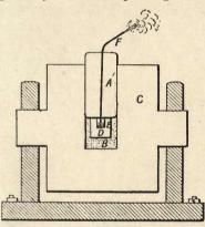
FIG. 38.—MORTAR FOR MEASURING THE BALLISTIC POWER OF EXPLOSIVES. A, Shot; B, Steel Disc; C, Section of Mortar (Cast-Iron); D, Wooden Plug holding Explosive (E); F, Fuse.
