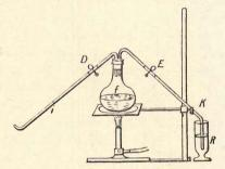
FIG. 336 .- DECOMPOSITION FLASK FOR SCHULTZE-TIEMAN METHOD.
