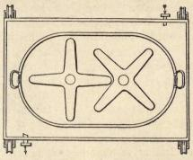
FIG. 105.—PLAN OF THE BOX CONTAINING THE EXPLOSIVE, IN M'ROBERTS' MACHINE. dynamite, it is at this point that the proper proportions of wood-pulp\* and potassium nitrate should be added,
