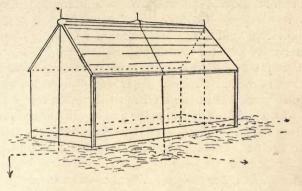
FIG. 4a.-GOVERNMENT SYSTEM OF LIGHTNING CONDUCTORS. FOR LARGE BUILDINGS.
