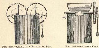
carried to a wringer, which forms the basket, and the acids removed. Finally, the cage is taken to a plunge tank, where the paper is removed from the cage by simply pulling out the central perforated cylinder B. Fig. 22 shows the nitrating pot, with its automatic
