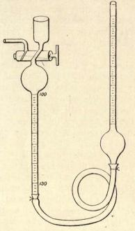
FIG. 30.-ORDINARY FORM OF LUNGE NITROMETER.
