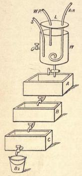
FIG. 8.—FILTERING AND WASHING PLANT. W, Lead Washing Tank; WP, Water Pipe; L, Lid; S, Nitro-glycerine from Separator; A B C, Filtering Tanks; B2, Indiarubber Bucket. be sent down a conduit to another building, in order to allow the small quantity of nitro-glycerine that has been retained in the water as minute globules to settle, if thought worth the trouble of saving. This, of course, will depend upon the usual out-turn of nitro-glycerine in a day, and the general scale of operations.
