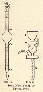
immediately closed. When the powder has dissolved—a process which may be hastened by warming the bulb very carefully —the thick solution is drawn into the nitrometer tube N, and the bulb rinsed several times with fresh acid, after which operation the analysis is proceeded with in the usual way.
