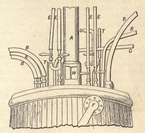
FIG. 5.—TOP OF NITRATOR. A, Fume Pipe; B, Water Pipes for Cooling; C, Acid Mixture Pipe; E, Compressed Air; G, Glycerine Pipe and Funnel; T, Thermometer; W, Window.
