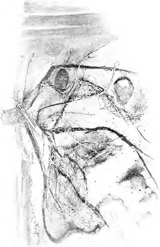
SECTIONAL VIEW OF STUMP SHOWING RELATIVE POSITION OF ROOTS AND EXPLOSIVE CHARGE
