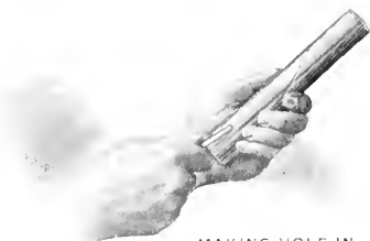
MAKING HOLE IN SIDE OF CARTRIDGE
