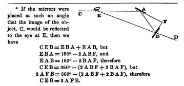
If the two mirrors be parallel to each other, and the angle formed by their planes equal therefore to zero, then
