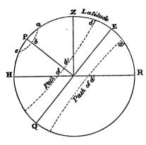
is made with a transit instrument or theodolite, carefully adjusted in the plane of the meridian, the readings of the vertical arc being noted at the time of the upper and lower transits of the star. These readings are then corrected for atmospheric refraction
