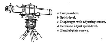
the telescope is attached to the bearing-frame, and the spirit-level firmly fixed to the tube of the telescope. The spirit-level is adjusted perpendicularly to the vertical axis of the instrument, by correcting half of the observed deviation by the screws d, and the other half by the parallel-plate screws e, until the telescope can be moved round in any direction without any material change taking place in the position of the bubble.
