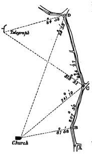
is adjusted and set to zero. the telescope having first been directed to the staff at A: the upper plate being then unclamped, the readings of one or more conspicuous objects in the neighbourhood are taken; and, lastly, the telescope being directed upon a staff fixed by an assistant at the forward station C, chosen at the next bend in the road, the upper plate is firmly clamped, and the forward angle read off. Proceeding from B to C, the line B C is measured
