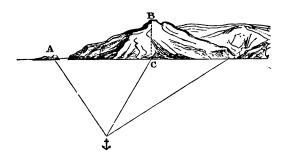
When the difference of elevation between the objects is considerable, an ideal vertical line (see sketch) may be drawn from the higher object downwards to an elevation corresponding to that of the lower object, and this, with some experience and correctness of eye, will give results sufficiently near to the truth.
