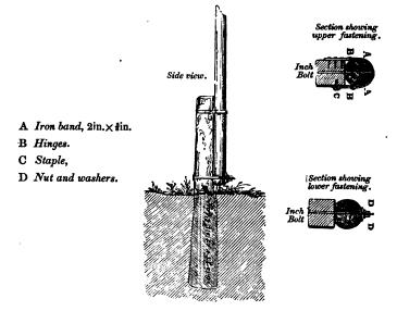
mast in its place, its lower end being fastened by a pin, round which it freely revolves as on a centre in a vertical
