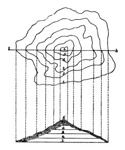
other. The marks thus supposed to be left on the hill being surveyed and drawn on the plan, would supply information more exact than a model in relief.'\*
