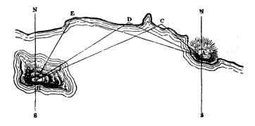
twice the sine of half the arc (see page 92). This reduction having been attended to, several intermediate points will also have been determined, if the observations at the primary stations have been made by day, as shown in the last figure, where A and B are the primary stations, from which the azimuthal bearings of the stations C, D, E, etc., have been observed.
