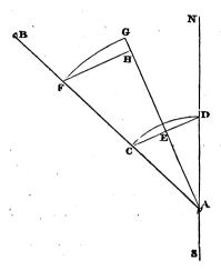
Let A B be the side of the triangle, the azimuthal angle of which has been ascertained with reference to N S, the meridian line. Take from an accurately divided diagonal scale, exactly five inches as a radius, and from A, as a centre, describe an arc C D; now the chord of an arc being equal to twice the sine of half the arc, the chord
