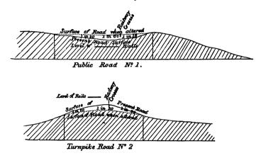
The cross section must show in figures, as well as by measurement, the present level and the intended level of the road.
