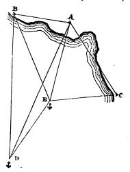
angles CEA, AEB—and it becomes, therefore, a fixed station with reference to D, from whence two angles are observed to three stations fixed in position.\*
