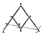
two sides, BD, BF, extended to double their length; the side DE, and the branch DA, are marked from D with successive divisions, DO being made to BO always in the ratio of DP to BC. Small sliding boxes for carrying a pencil, or a tracing point,
