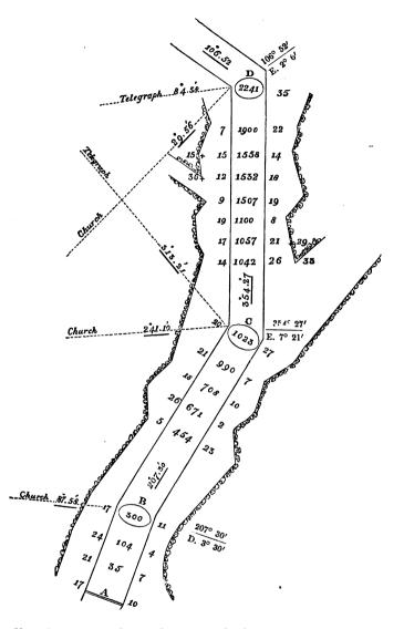
direction upon those that precede it, errors will, except under favourable circumstances, be introduced into the work. The different parts of a traverse should therefore be referred to certain accurately fixed points, and any errors thus discovered may, if small, be corrected and allowed for in the plotting.
