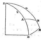
Let A and B be the objects observed, and H R the projections of A and B. on the plane of the horizon, required the arc H R. Observe the angular elevations A H, B R, as explained in the description of the Sextant.
