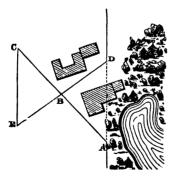
ible point on A D, measure a line D B E, making B E equal to B D, then C E will be equal to A D, the distance required. This method is inapplicable if the line has not been previously ranged and determined by signals fixed beyond D, and visible from it.
