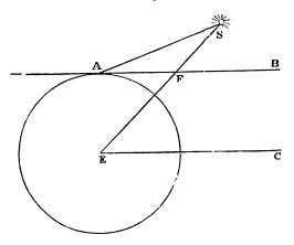
earth's surface, S the sun, A B the artificial horizon, E C the true horizon, then the parallax is the difference be-
