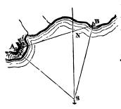
the position and bearing of the points on shore are given, with respect to each other. For, let A and B be two objects on shore, fixed in position with reference to one another and to their bearing with the meridian; and let S be the position of the ob-
