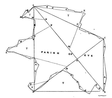
'The two main-lines which I should recommend to be measured through it are marked A B, and C D.
