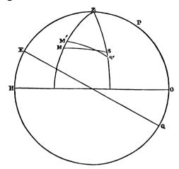
*Example.*\*—On May 4th, 1838, at 10<sup>h</sup> 38<sup>m</sup> 12<sup>s</sup> by chronometer, the following observations were taken, in latitude 51° 23'40' north, to find the longitude.
