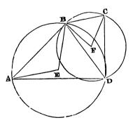
*Example.* Let the three objects on shore, A, B, C, be fixed in position; and let the angle subtended at D by A B be equal to  $50^{\circ}$ , and the angle subtended by B C be equal to  $40^{\circ}$ ; to find the point D by construction. Subtract double
