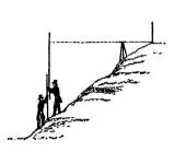
When levelling over a steep slope, or when the level has been fixed so that the staff falls below the range of the horizontal ray, much time may be saved by having the second staff held at a definite distance up the first, so that
