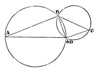
The first of these consists in a geometrical construction. Let A, B, and C, be the three stations, and D the position of the observer, at which the angles A D B, B D C, have been measured.
