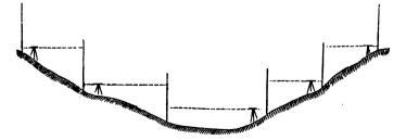
rising on the opposite side; this arrangement avoids the necessity of taking the sights inconveniently close to one another. The alternation also tends, by a compensation of errors, to correct in the final result the effect of any error that might be due to imperfect adjustment in the line of collimation.
