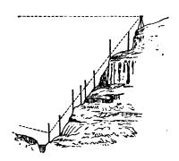
the proper reading of the staff, and owing also to the great number of readings required in a short horizontal distance. With the theodolite, on the contrary, it is sufficient to place the instrument at the top or bottom of the ravine, and take the differences of level as
