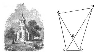
When the instrument is placed at the base of a tower or high permanent object, the centre of which is the true vertex of the triangle, it sometimes happens that the centre of the station cannot itself be seen, but the direction of that centre from the axis of the instrument is required for the purpose of measuring the angle A D C. The direction of the centre is found as follows :---
