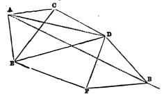
of the three angles CDE, EDF, and FDB, and you have the angle ADB; with this angle and the two sides, AD and DB, compute the angle DBA; this is the difference between the bearing of A from B, and that of D from B. The latter is known, or can be directly observed; whence the former is deduced.
