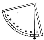
independently of its use in measuring vertical angles, it is of great assistance in tracing level lines in sketching the contours. The instrument sold under this name is made with a spirit level; but the substitute as described above answers the purpose equally well, and moreover, from its being made merely of pasteboard, fits into the pocket of the sketching portfolio.
