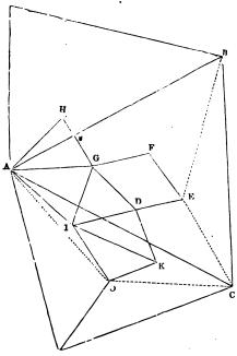
thus the connection between the three classes of triangles was established, and the positions of many of the minor stations, which had been determined by calculation from a series of small triangles, were checked by being made the vertices of larger triangles, based upon sides of those of the second order.
