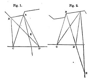
radius A B; and the distance required for the battery can therefore be laid off on the ground by increasing or diminishing the length of this line A E.
