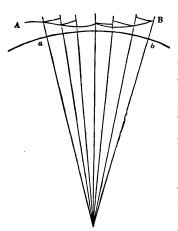
nearly enough), and h the elevation, the measured lengths must be multiplied by the fraction  $\frac{r}{r+h}$ or  $1\frac{h}{r}$ , or they must be diminished by the part  $\frac{h}{r}$  of the whole. If the surface slopes uniformly, the mean height may be taken; if it is very irregular, it may be divided into several parts."
