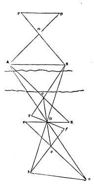
A right angle<sup>\*</sup> can often be laid off when no means of measuring other divisions of the circle are at hand. The distance A B can then be thus obtained :—
