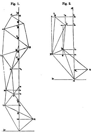
being short), or more correctly to X', the point of intersection with this meridian of the *parallel drawn through* L becomes the distance to be attained by calculation. The length of A B, or of any other side, is first accurately determined with reference to some measured base, and the angles at the vertices of all the triangles observed with the most rigid accuracy; and after the necessary corrections for spherical excess have been made, with the reductions to the
