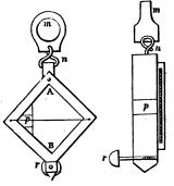
turned round, and the observer, placed between it and the wall, with his back to the latter, notes the spot where the *image of his eye* coincides with the reflected wall above or below the former mark. The mean distance between these two points is assumed and marked, and by turning the screw r, the centre of gravity of the mirror is altered until the image of the eye coinciding as before with the silk
