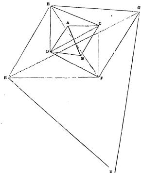
already stated that the sides of the principal triangles should increase as rapidly as possible from the measured base. Theaccompanying sketch will show how this is to be managed without admitting any ill-conditioned triangles.
