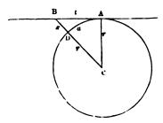
radius, 2r may be substituted for (2r + x), and the arc a for the tangent t; 2rx then becomes  $= a^2$ , and  $x = \frac{a^2}{2r}$ , which, assuming the mean diameter of the earth at 7916 miles, gives x = 8.004 inches or 667 of a foot for one mile; which quantity increases as the square of the distance. Or otherwise,
