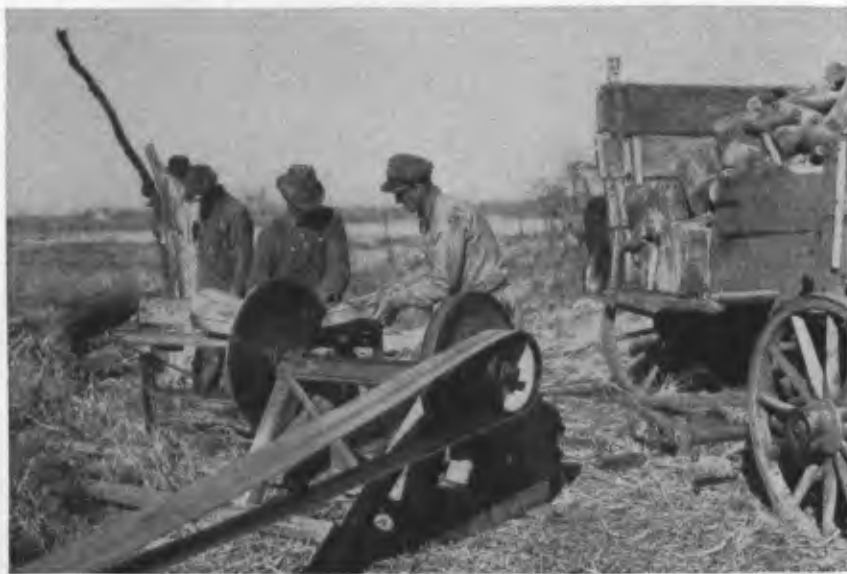
FIGURE 8.—Working up Osageorange into stovewood with a buzz saw, near Hutchinson, Kans. Throwing the short lengths immediately into the wagon saves labor. The saw, belt pulley, and flywheel should be provided with safety guards.
