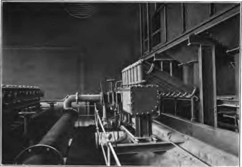
FIG. 13.—Arrangement of pipes over the retort bench for collecting the first fluid distillates.
