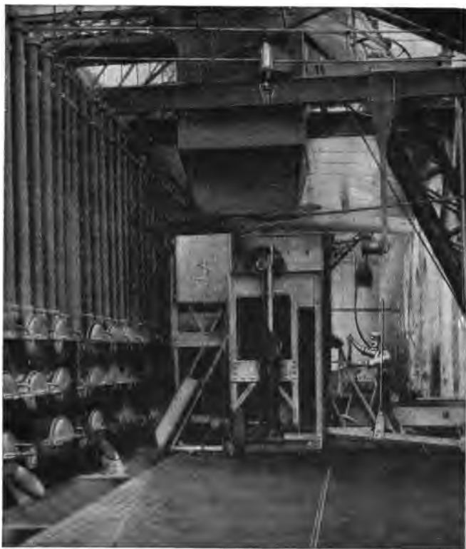
FIG. 9B.—West's combined charging and drawing machine, driven by compressed air.
