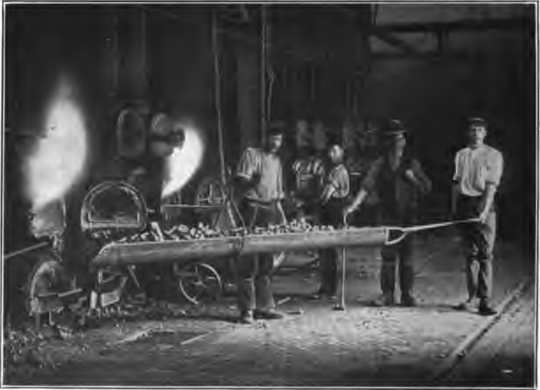
FIG. 8.—Hand retort charging machine (Biggs-Wall).
