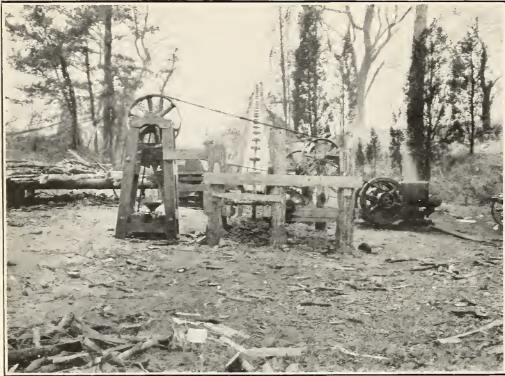
FIG. 1.—BUZZ SAW, POWER SPLITTER, AND CONVEYOR, SET UP AT DOVER, MASS.
