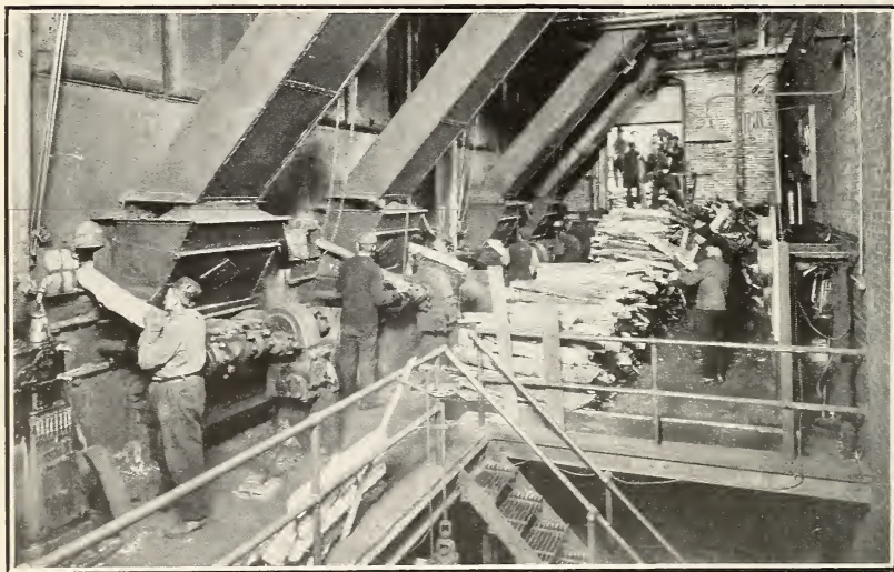
FIG. 2.—FIRING WITH WOOD FUEL; FURNACES IN A NEW ENGLAND FACTORY EQUIPPED WITH AUTOMATIC STOKERS FOR COAL.
