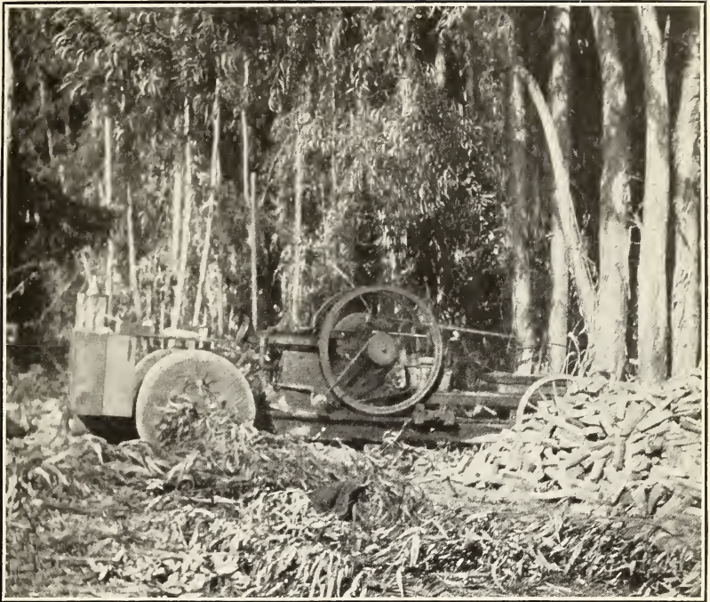
FIG. 1.—SAWING BLUE GUM (EUCALYPTUS) WOOD WITH GASOLINE ENGINE. Rate 1\frac{1}{2} to 2 cords per hour. Santa Fe Springs, Cal.
