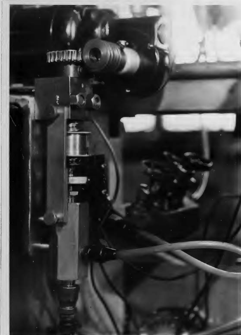
Figure XII - Control Valve and Flowmeter Block
