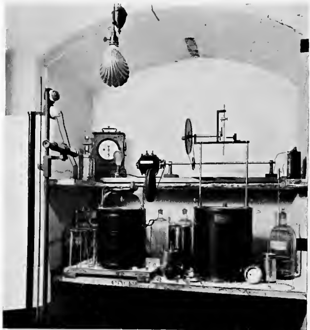
Fig. 62.—Bomb Calorimeter, with Stirring Gear driven by Electric Motor.
