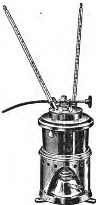
FIG. 45.—Tag closed tester for flash point of oils.
