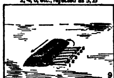
9 Halving by alternate shovel method. Shovelfuls 1, 3, 5, etc., reserved as A; 2, 4, 6, etc., rejected as B.
