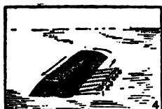
4 Halving by alternate shovel method. Shovelfuls 1, 3, 5, etc., reserved as A; 2, 4, 6, etc., rejected as B.
