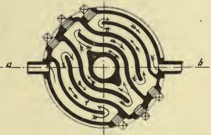
Fig. 87. SYMON-HOUSE BURNER AND VAPORIZER
