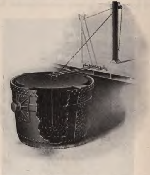
Fig. 80. Ladle-Drying and Heating Oil Burner.
