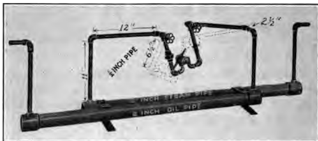
Fig. 48. Burner for Up-Draft Kiln.
