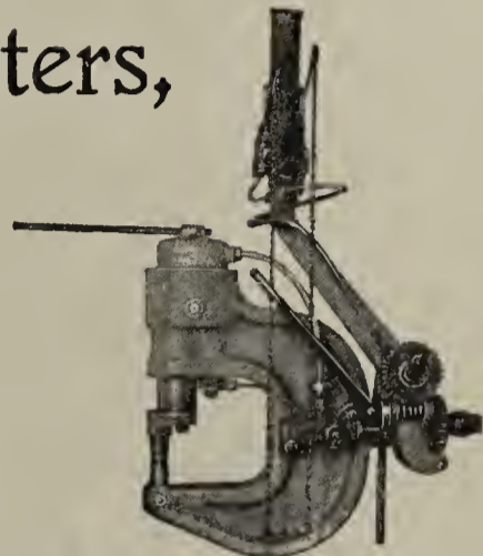
Portable Hydraulic Riveter and Hydraulic Lift.
