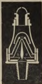
Fig. 16.—Peebles's Needle Governor Burner.
