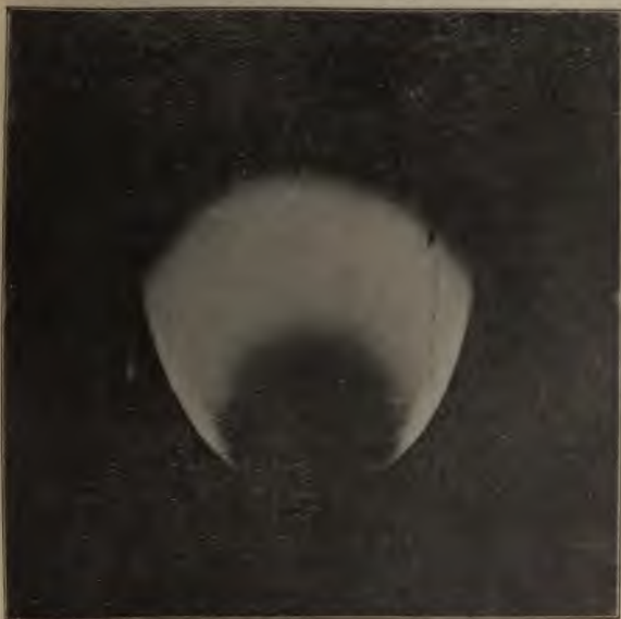
Fig. 19 (b).—Union-jet or fish-tail flame.
