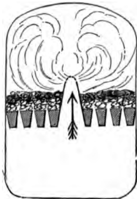
Fig. 29.—Air through orifices in the fireplace.
