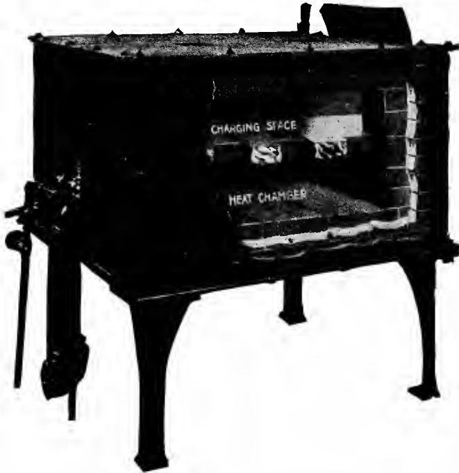
Fig. 147. View showing the heat in an indirect-fired furnace passes from the heat chamber through graduated heat ports.
