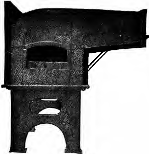
Fig. 45. Furnace with front casting removed to show special shaped brick lining.
