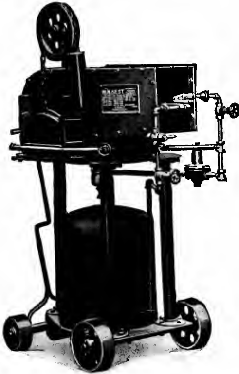
Fig. 216. Portable, self-contained outfit for rivet heating, etc.
