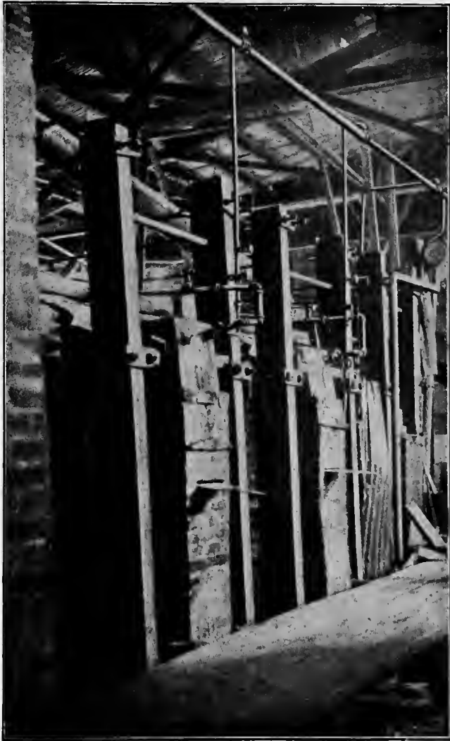
Fig. 303. Old type glass melting furnace, practically obsolete to-day. Size in the bath, 14 feet. by 18 ft.
