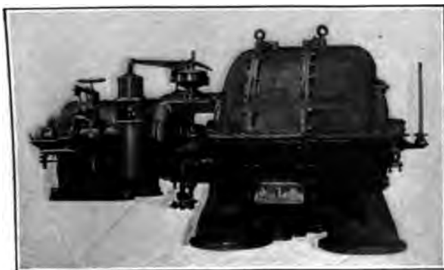
Fig. 85. Exhausters Driven by Steam Turbine
