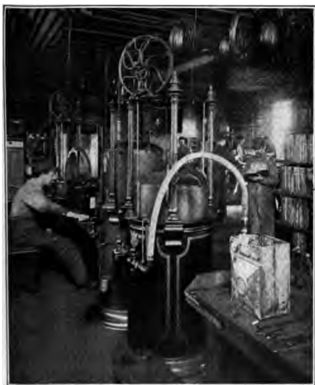
Fig. 298. Meter Provers and Meter Under Test
