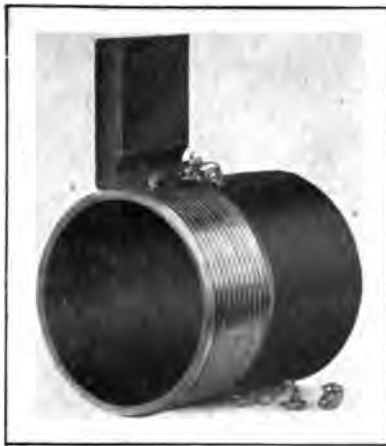
Fig. 249. Cutting Thread on Steel Pipe
