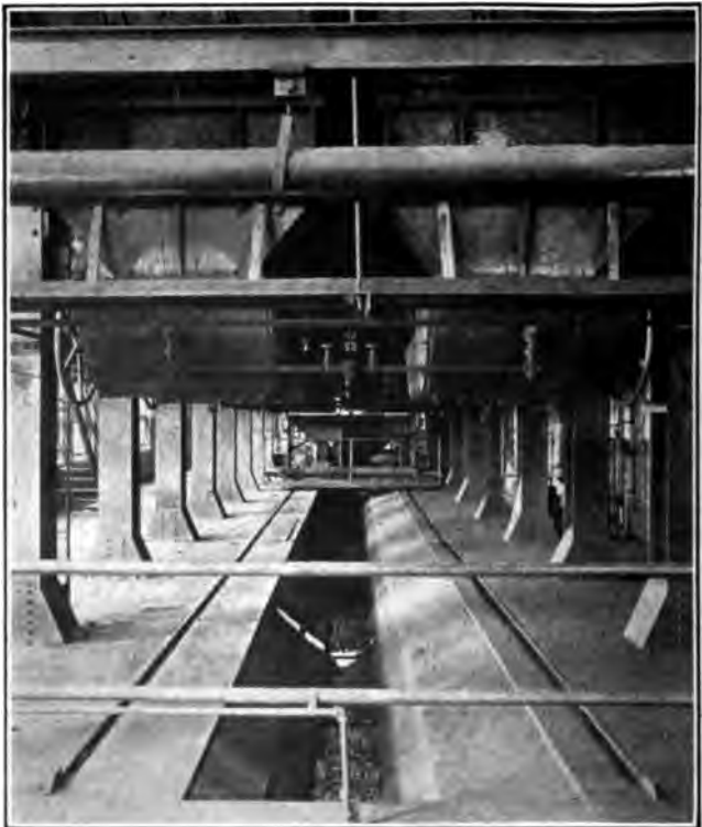
Fig. 18. Vertical Retort Coke Discharge Provisions
