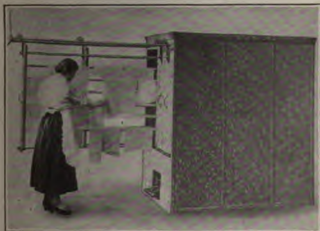
Fig. 7. Gas-heated Laundry Dryer
