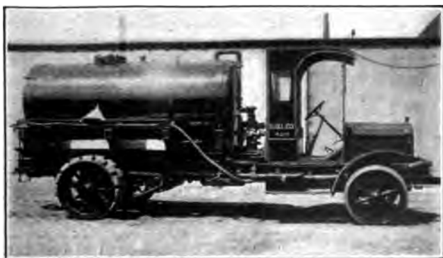
Fig. 138. Power Pump on Motor Drip Wagon
