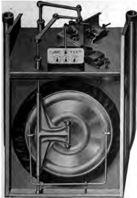
Fig. 288. Front and Top Removed From Tin Meter
