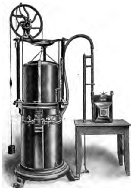
Fig. 300. A Typical Meter Prover
