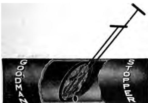
Fig. 333. Main Stopper in Position
