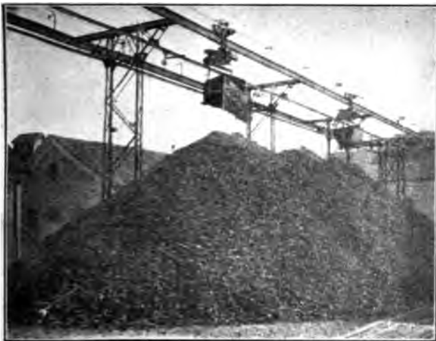
Fig. 148. Trolley Automatically Transports Fuel
