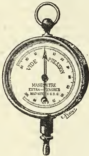
Fig. 1.—DIAL-PLATE GAUGE FOR DETERMINING GAS PRESSURES AND CHIMNEY DRAUGHTS.
