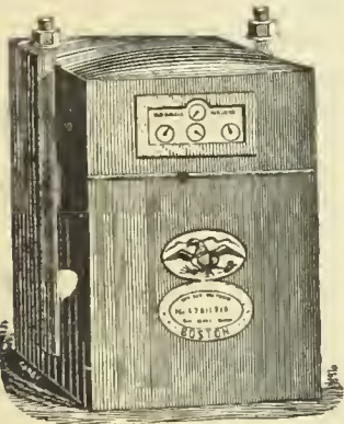
Dry Gas Meter.
