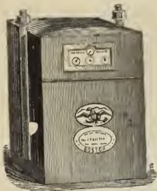
Dry Gas Meter.
