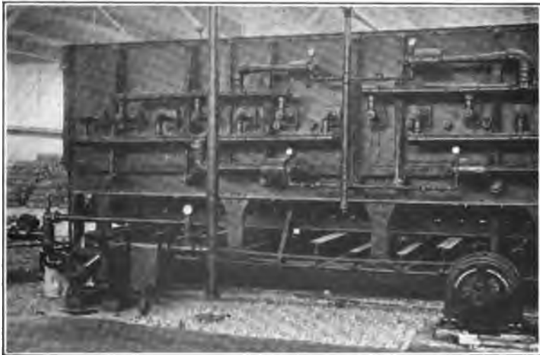
FIG. 357. —Automatic surface combustion shell-drawing furnace, Pawtucket, R. I. City gas used as fuel.
