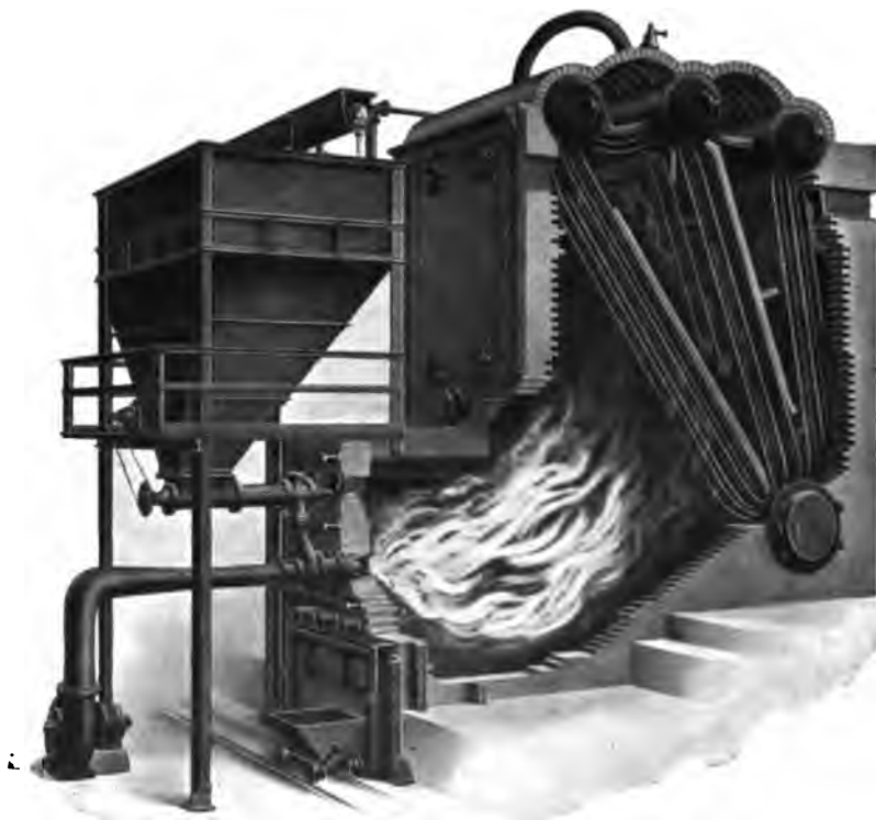
FIG. 168.—Stirling boiler equipped for firing with pulverized coal, Fuller-Lehigh system.
