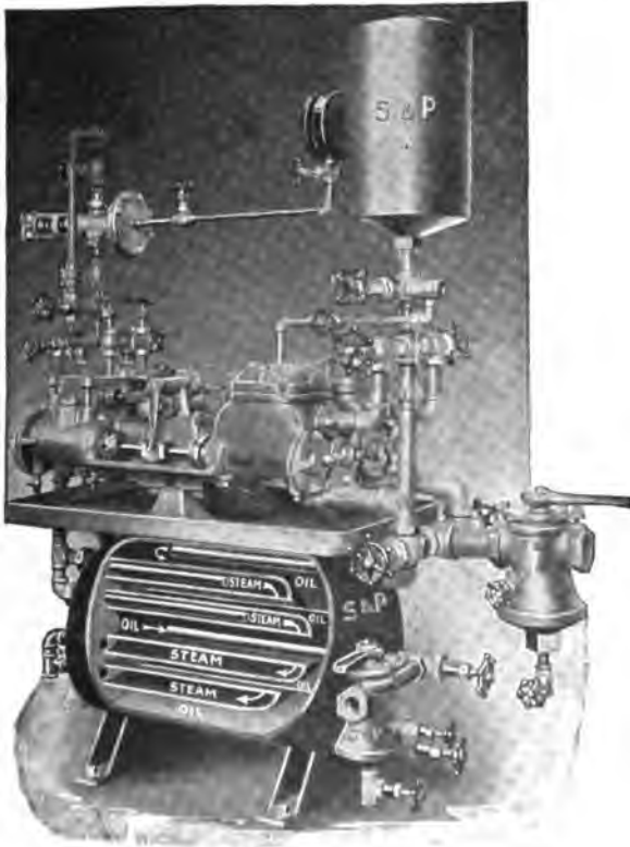
FIG. 205.—The Staples & Pfeiffer self-contained, self-cleaning, self-governing, automatic oil-pumping, heating and filtering system.
