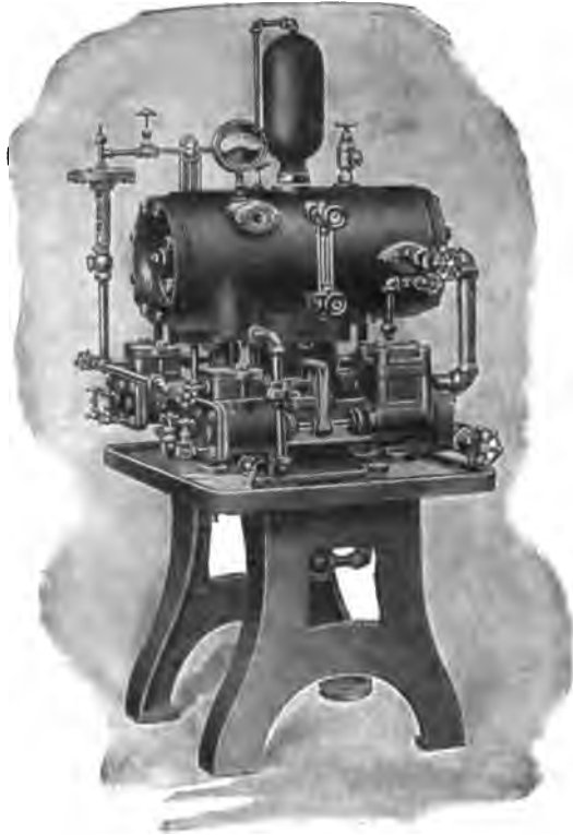
FIG. 208.—A fuel oil-pumping outfit manufactured by the Worthington Pump and Machine Company, of New York, N. Y.
