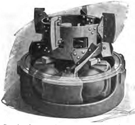
FIG. 166.—Rotating element of Fuller mill with balls, pushers, plows and fan blades.
