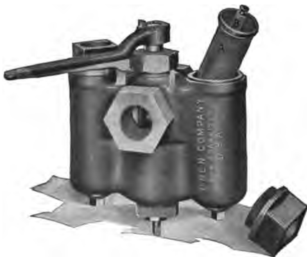
FIG. 219.—The Coen duplex oil strainer. A and B show the two parts of the strainer basket; the combined area of the perforation of the total baskets is from 6 to 10 times the cross-sectional area of the pipe.
