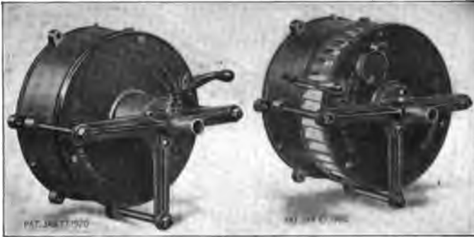
FIG. 216.—The Coen air register, which is built in 2 sizes, 18 in. and 22 in., respectively, for marine and land boiler installations. This register is designed to give an intimate mixture of the air supply and spray with a minimum of draft restriction.
