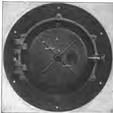
FIG. 271.—Coen firing front for Scotch marine boilers. This swing-type firing front has been simplified somewhat from that shown in the preceding figure.
