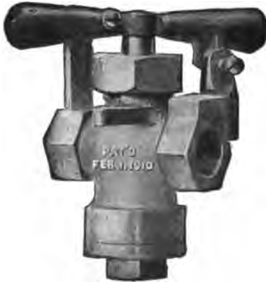
FIG. 224.—The W. N. Best "Calorex" oil regulating cock. This regulating cock has a v-shaped, knife-edge, opening in the plug which not only has a shearing action on heavy liquid fuels, but enables the operator to secure the desirable adjustment.
