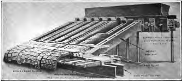
FIG. 192.—Riley self-dumping underfeed-stoker. Perspective view of a nine-retort stoker partially assembled, showing independence of unit parts.
