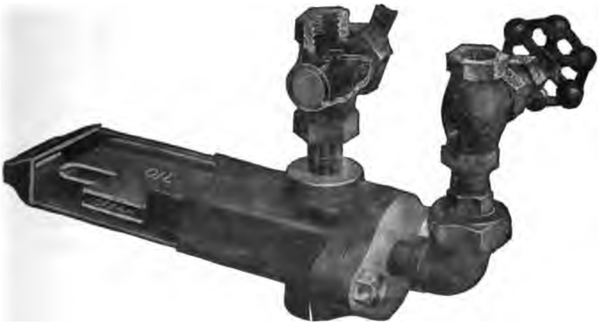
FIG. 222.—Staples & Pfeiffer gravity type crude oil burner, for oil pressures from 1 lb. up, or 2 ft. elevation up, and for crude oil with steam atomizing.
