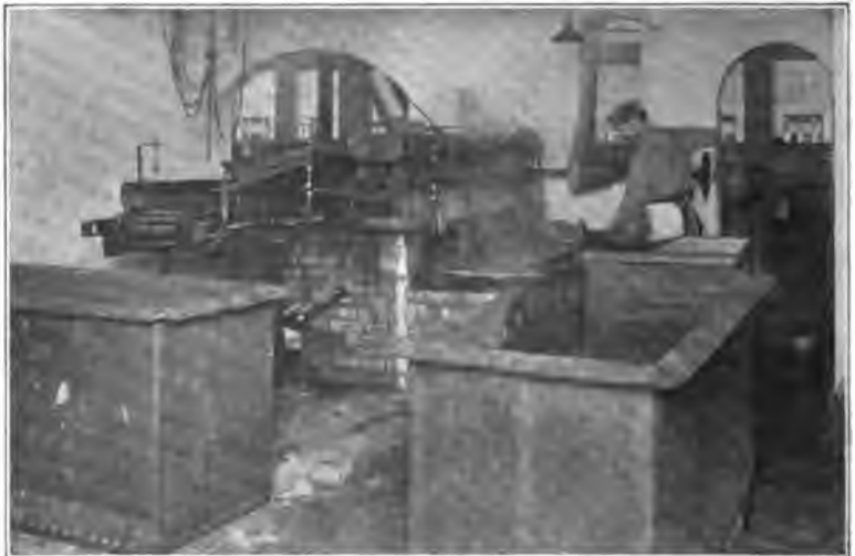
FIG. 359.—Surface combustion tinning pot—one of a battery of 40. Coke-oven gas used as fuel.
