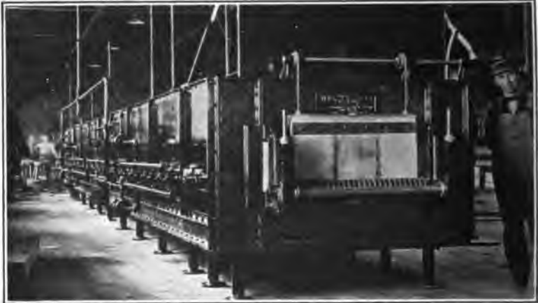
FIG. 354.—Surface combustion wire patenting furnace—delivery end.
