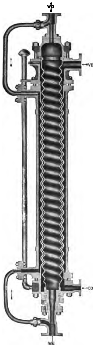
FIG. 213.—The film oil heater manufactured by the Schutte & Koerting Company, Philadelphia, Pa.
