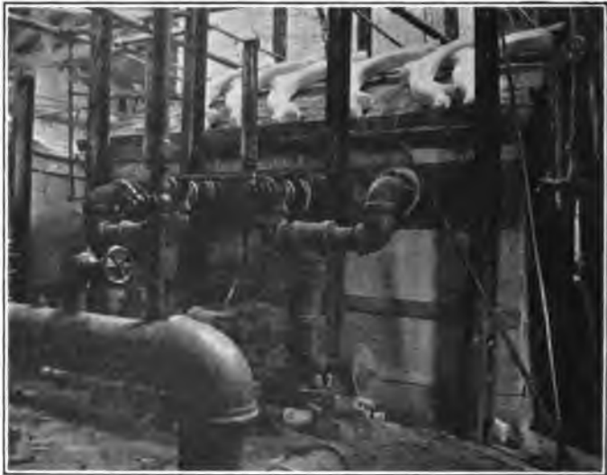
FIG. 347.—Surface combustion day tank for melting very refractory glass. Natural gas is used as fuel.
