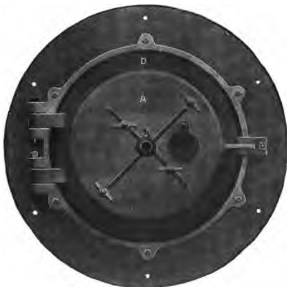
FIG. 266.—The latest Coen firing front for oil-fired boilers. A is an adjustable damper which controls the air supply to the interior of the firing front; and D is a hinged part which allows it to be swung open; access to the furnace is available at any time without disconnecting or removing any parts.
