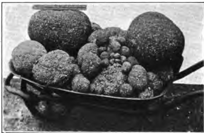
FIG. 85.—Clinker balls discharged from a gas producer of the horizontal rotary type.
