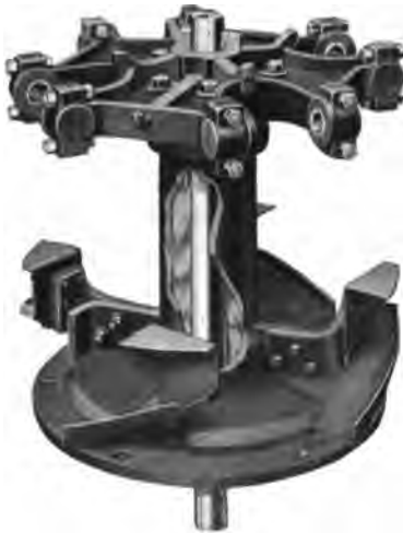
FIG. 125.—Rotary element of Raymond mill with spider and plows.
