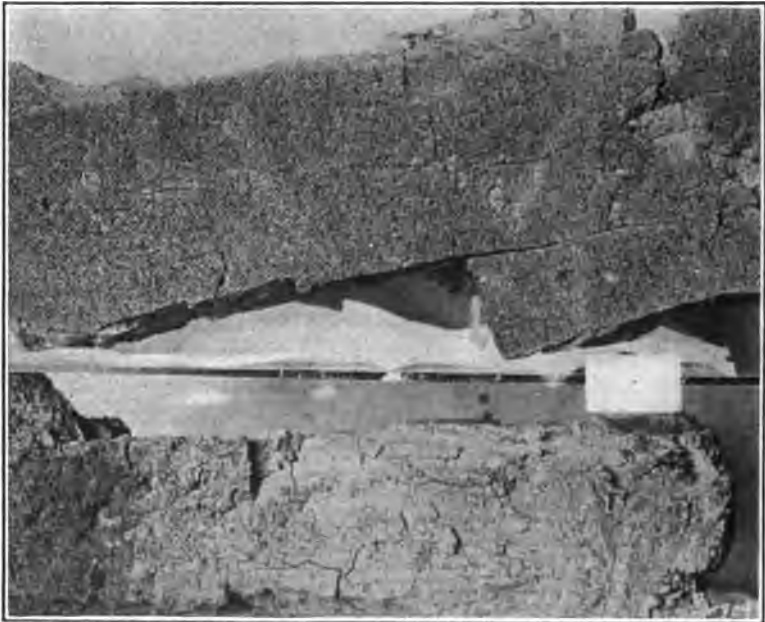
FIG. 10.—Natural surface and longitudinal section of by-product coke.
