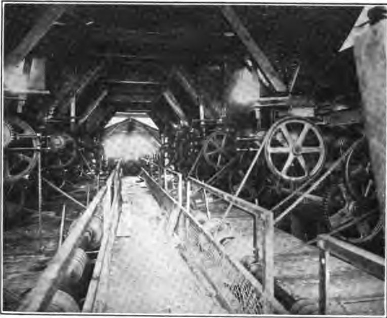
FIG. 94.—Arrangement of automatic feed of primary retorts of carbocoal plant of Clinchfield Carbocoal Corporation, South Clinchfield, Va.
