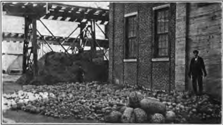
FIG. 84.—Clinker balls discharged from a gas producer of the horizontal rotary type.
