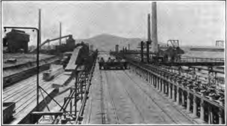
FIG. 31.—Top of battery of 106 Koppers ovens, Bethlehem Steel Company, South Bethlehem, Pa.
