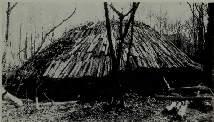
Covering the pit with leaves and dust
