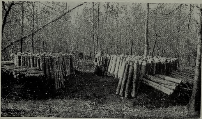
Filling a hearth with lap-wood and billets
