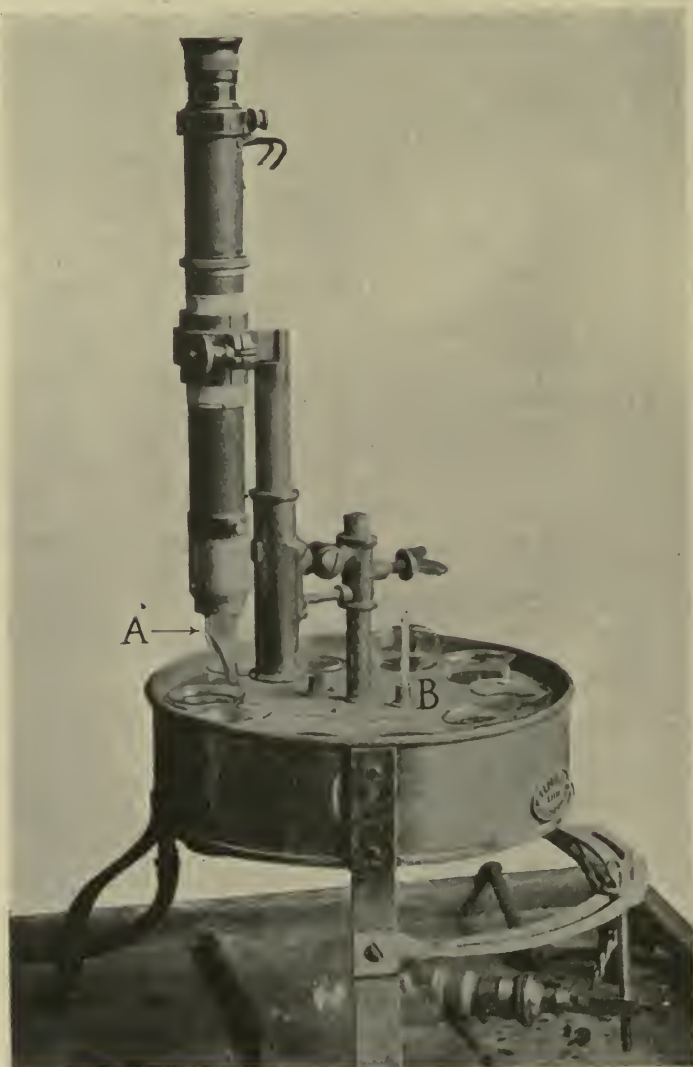
FIG. 46.—IMMERSION REFRACTOMETER, WITH ROTATING WATER-BATH. A , prism, which dips into the liquid in the glass beneath; B , bath with thermometer.
