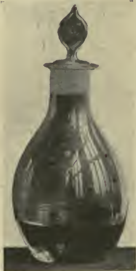
FIG. 36.—FLASK USED FOR ACETONE AND BROMINE TESTS OF WOOD-NAPHTHA.
