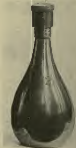
FIG. 37. — SILVER PRESSURE FLASK. Used for determining esters in wood-naphtha.
