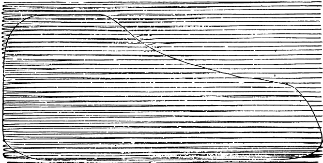
FIG. 81.—Diagram taken with Wayne Indicator.
