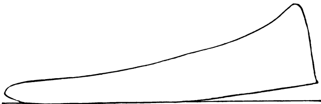
FIG. 41.—Indicator Diagram from Fielding and Platt's Engine, running at nearly full load.
