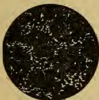
FIG. 82. — B Series; tensile strength 36,600 pounds per sq. inch; magnification 120 diameters.
