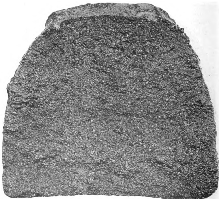
FIG. 183.—Holwell, No. 4, Foundry.
