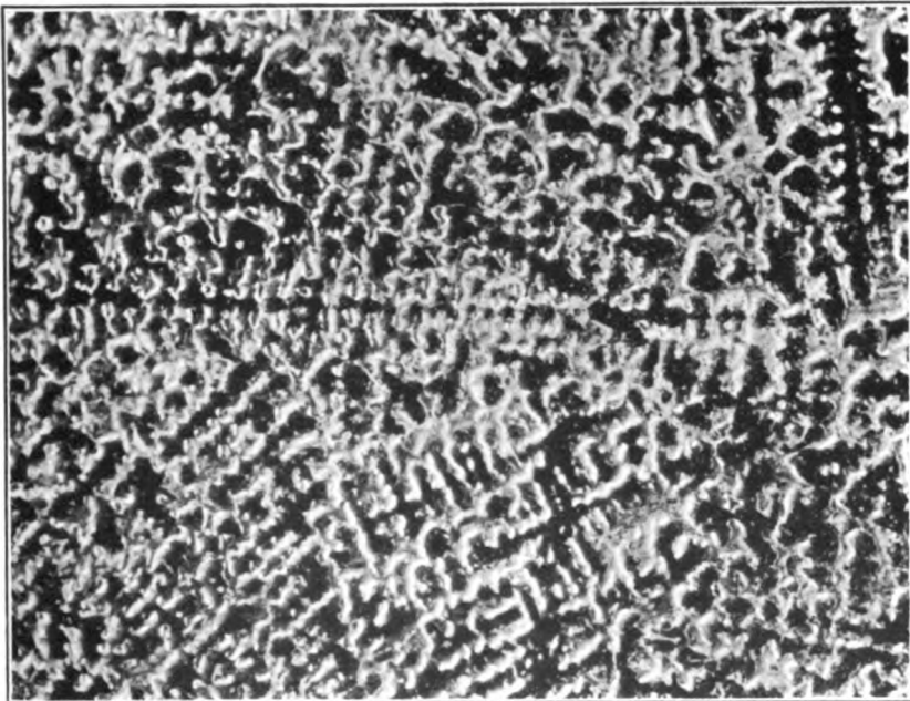
FIG. 231.—Structure of Pure Gun Metal. \times 58 . Maximum Stress, 9.5 tons per square inch. Elongation, 2.8 per cent. on 2 inches.
