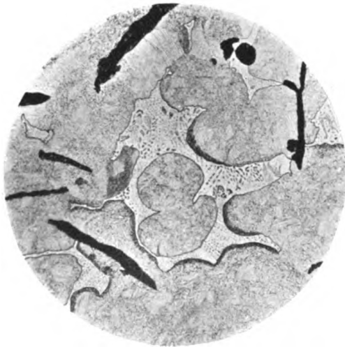
FIG. 237.—Grey Cast-iron. (Section prepared by Dr. Sorby in 1864.) \times 460 .
