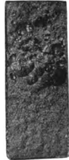
FIG. 173.—Fracture showing Blowholes.
