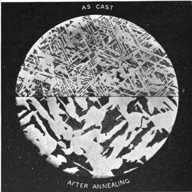
FIG. 206.—Structure of Steel Casting. \times 66 .
