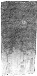
Fig. 152.—Chill Test Fracture.
