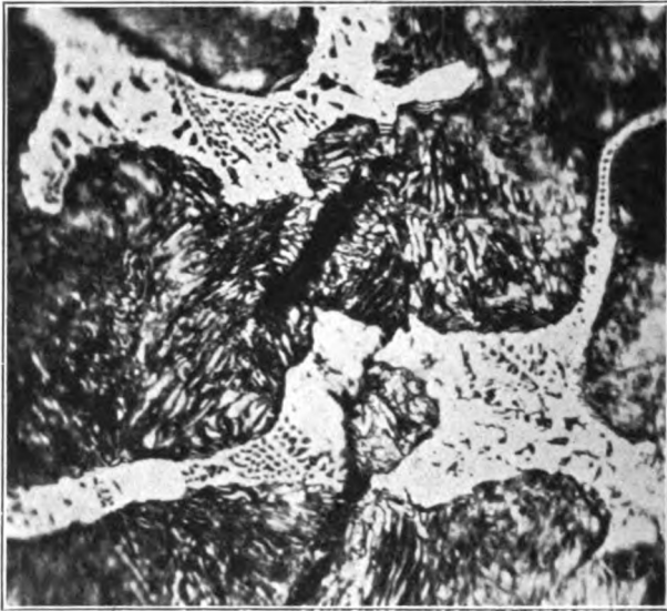
FIG. 241.—Phosphide Eutectic. \times 1000 .
