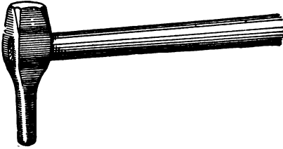
Fig. 51. Punch for Heavy and Fast Work
