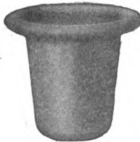
Fig. 204. Cast-Iron Pot Used for Lead Pot
