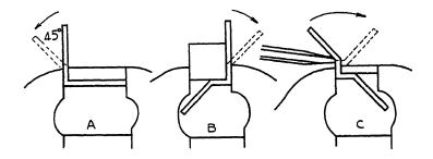
Fig. 57. Shaping a hack-saw-frame guide
