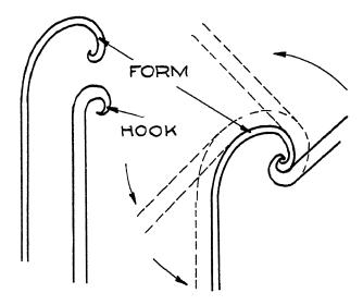
Fig. 36. Bending a scroll over a scroll form
