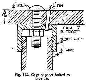
3. Shape the curve which is to support the cage, as in the drawing.
