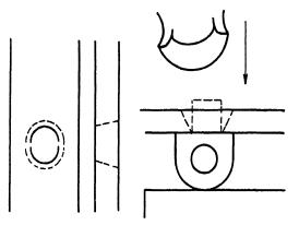
Fig. 78. Riveting the support to the back
