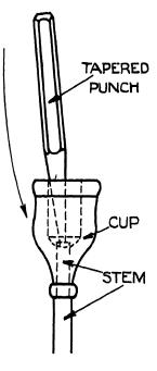
Fig. 92. Riveting the cup to the stem
