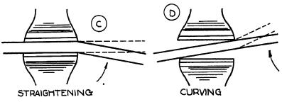
Fig. 25. Making bends in a vise
