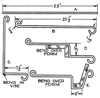
Fig. 75. Making bends in legs for magazine basket
