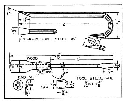
Fig. 53. Top: Wrecking bar Bottom: Screw driver
