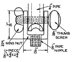
Fig. 116. Method of attaching lamp socket to pipe
