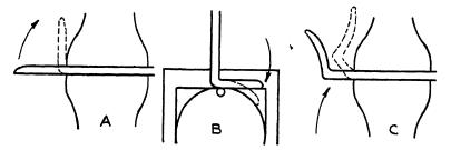
Fig. 91. Bending the feet of the log holder
