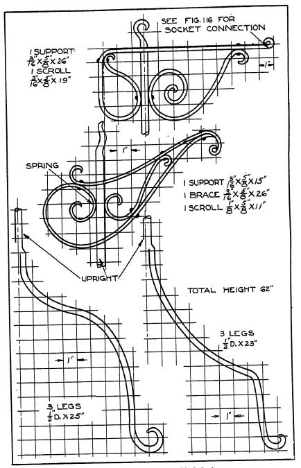
Fig. 120. Bridge lamps, welded design
