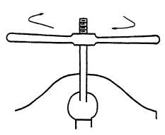
Fig. 46. Using a thread-cutting die
