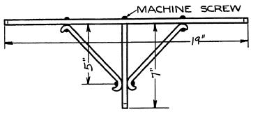
Fig. 69. Braces riveted in place
