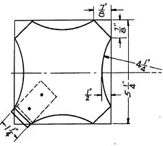
Fig. 107. Pattern for base and four feet
