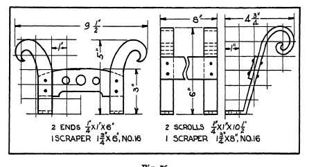
Fig. 76 Foot scraper, goat's-horn design Foot scraper, scroll design
