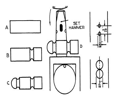
Fig. 60. Steps in making a hammer head
