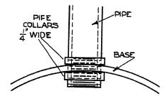
Fig. 104. Fastening pipe to base
