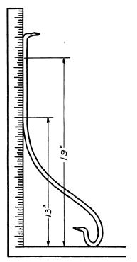
Fig. 112. Leg placed inside of carpenter's square
