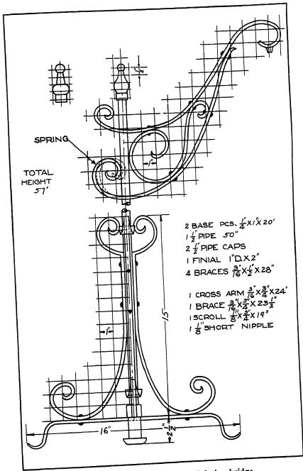
Fig. 118. Bridge lamp with scroll-design bridge
