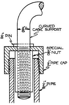
Fig. 114. Curved cage support carried down through cap
