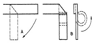
Fig. 62. Folding over ends of cross strips
