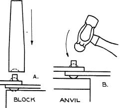
Fig. 43. Riveting
