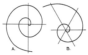
Fig. 34. Developing spiral curves
