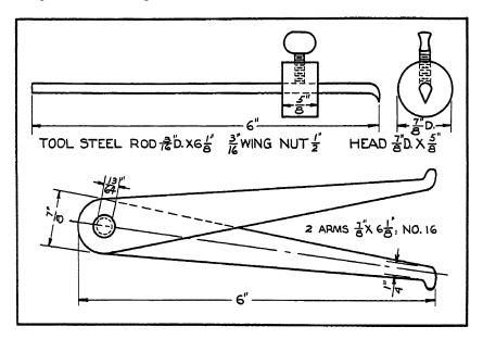
Fig. 52. Top: Combination marking gauge and depth gauge Bottom: Firm-joint calipers
