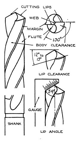
Fig. 41. Details of metal-working drill
