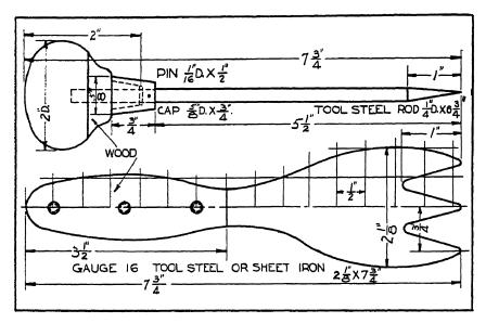
Fig. 55. Top: Ice pick Bottom: Ice scraper
