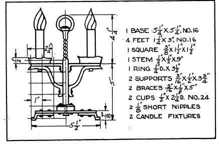
Fig. 106. Two-bulb lamp, with ring ornament
