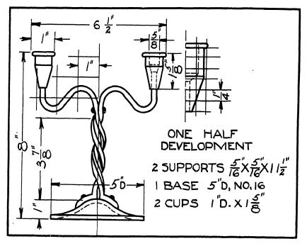
Fig. 97. Two-arm candlestick, twisted design
