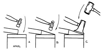
Fig. 19. Drawing a taper on a square bar
