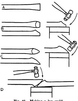
Fig. 49. Making a lap weld
