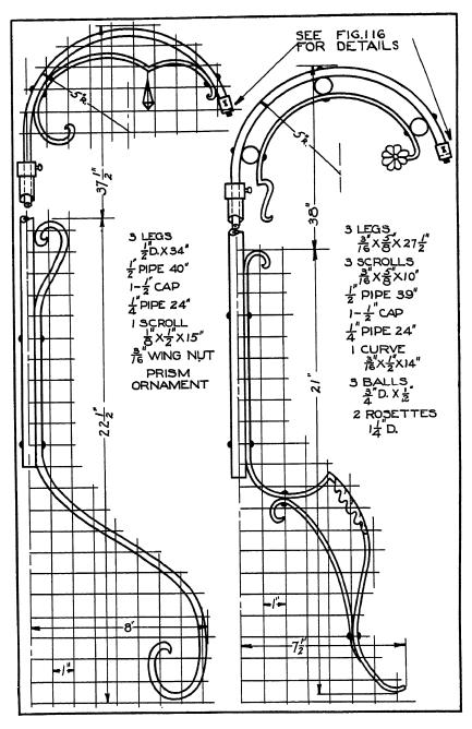
Fig. 115 Bridge lamp with prism ornament Bridge lamp with rosette ornament 2. The 1/4-in. pipe must be heated, and bent carefully over a simple form. Carelessness will cause the weld in the pipe to open up.
