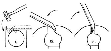
Fig. 64. Steps in bending the feet of the stool
