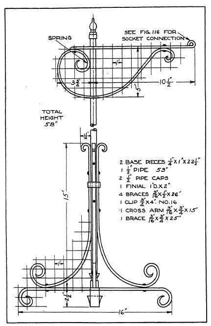
Fig. 117. Bridge lamp with spring-design bridge
