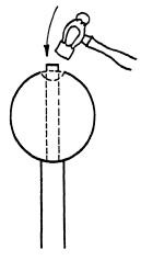
Fig. 85. Riveting the ball in place
