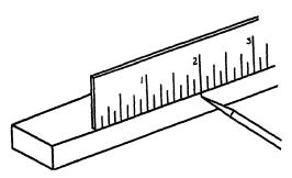
as in Figure 8, in order to insure accurate measurements. Because of its sharp point, a scratch awl will make a mark about  $\frac{1}{64}$ -in. wide, which is much more accurate than a mark made with a lead pencil.
