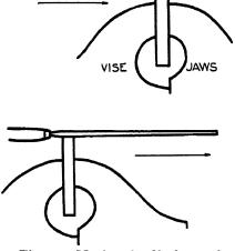
Fig. 17. Moving the file forward for the cutting stroke
