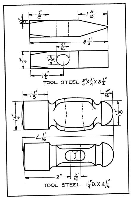
Fig. 59 Tone Diveting hammer head.—Bottom: Machinist's-hammer head
