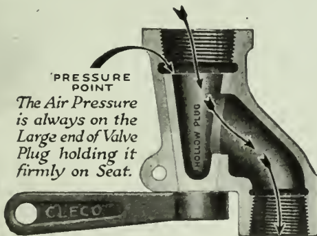
Cross-Section of Cleco Valve
