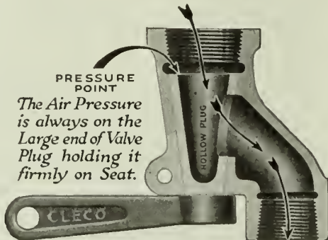
Cross-Section of Cleco Valve
