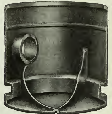
Auto Piston 20% Steel Cast 5/32-inch thick— machined to 3/32
