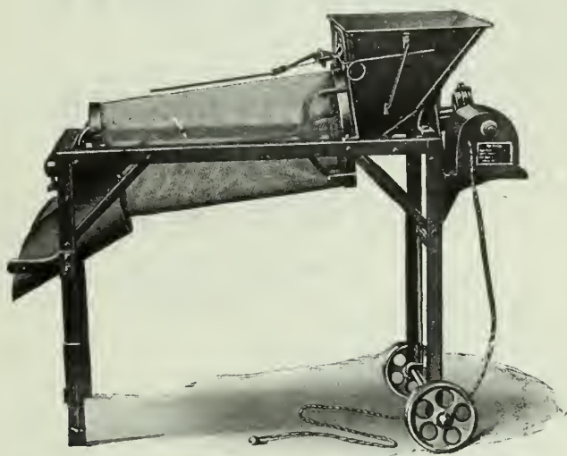
The Grand Rotary Sand Riddle is built with cranks for hand power; pulley for belt power, or \frac{1}{4} h.p. a.c. or d.c. motor for electric power.
