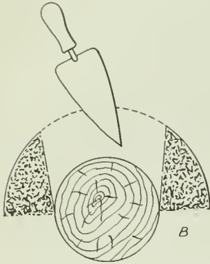
DIGGING AWAY SAND TO ALLOW PATTERN TO BE TAKEN OUT.
