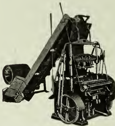
SIDE VIEW OF AUTOMATIC MACHINE SHOWING ELEVATING CONVEYOR.
