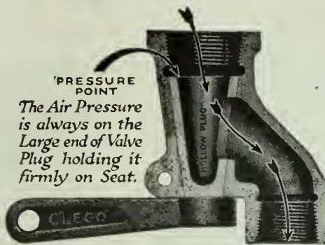
Cross-Section of Cleco Valve
