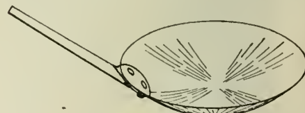
FIG. 3—BOTTOM ON WHICH FIRE CLAY CRUCIBLE IS BUILT.
