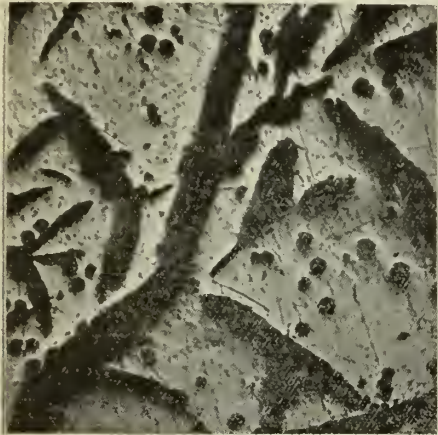
FIG. 2—MICROGRAPH SHOWING FREE CARBON IN CAST IRON.
