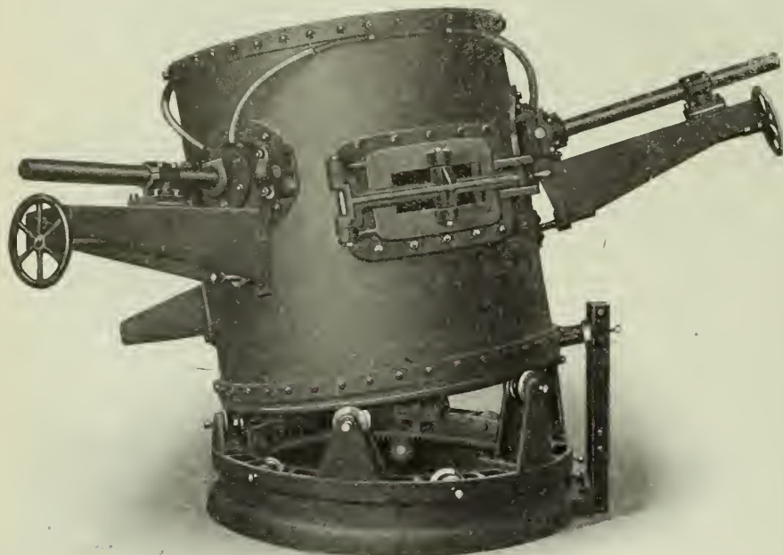
NOTE THE BASE AND ROLLERS WHICH GIVE THE FURNACE THE GYRATORY MOVEMENT
