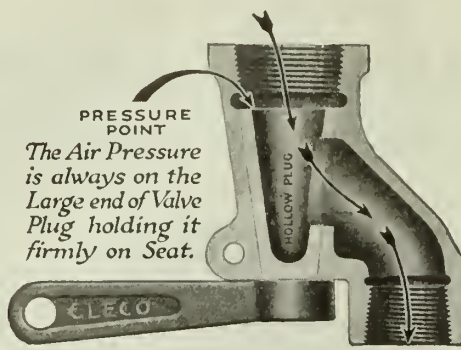
Cross-Section of Cleco Valve
