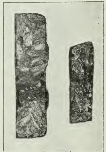
FIG. 14—FRACTURE DUE TO LOW SILICON ACCOMPANIED BY LOW CARBON AND MANGANESE.
