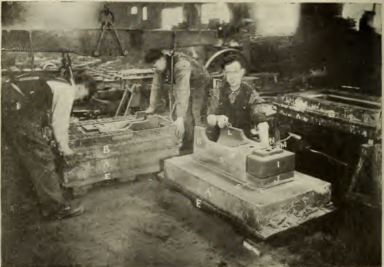
FIG. 2—TO THE RIGHT DRAG, WITH CORES COMPLETE. TO THE LEFT, CHEEK BEING LOWERED INTO PLACE.
