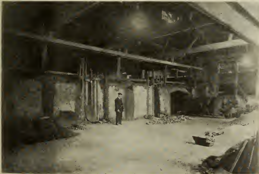
FIG. 6—ANNEALING OVENS, SHOWING ENGINE PLACING LOAD OF CASTINGS TO BE ANNEALED
