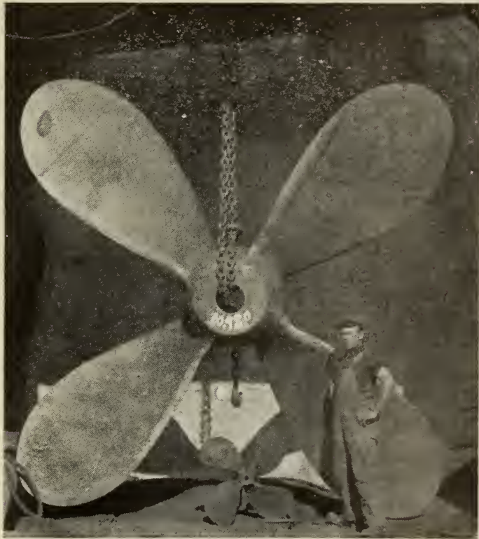
FIG. 1. SHOWS FOURTEEN-FOOT TEN-INCH PROPELLOR WEIGHING FIVE AND ONE-HALF TONS. NOTE THE SMALL ONE UNDERNEATH.
