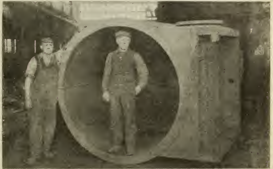
14,200 LB. SEMI-STEEL MARINE CYLINDER, MADE BY THE CANADA MACHINERY CORPORATION, LIMITED, GALT, ONT.
