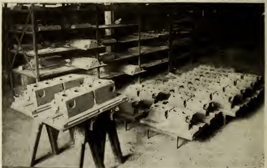
FIG. 2. SHOWING CORES WHICH ARE MADE ON THE JOLTING MACHINE.
