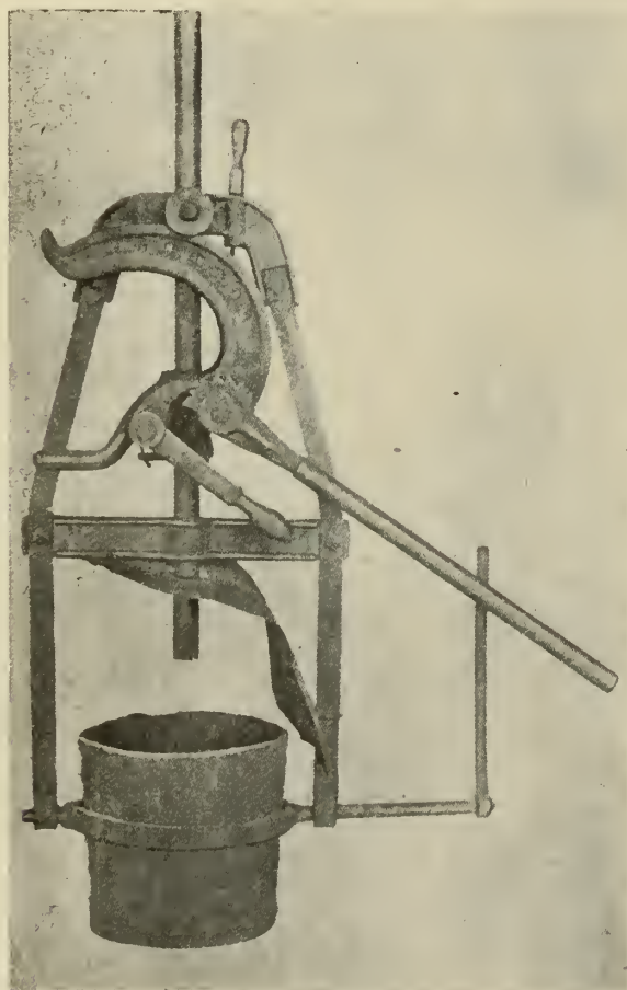
FIG. 1—A POURING DEVICE SUITABLE FOR HANDLING 350 POUNDS OF IRON
