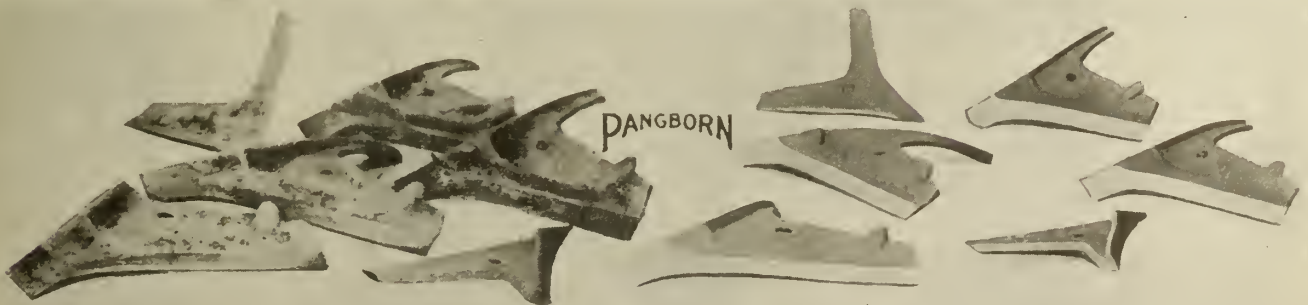
PLATE 15—PLOW POINTS, BEFORE AND AFTER CLEANING IN REVOLVING BARREL MACHINE
