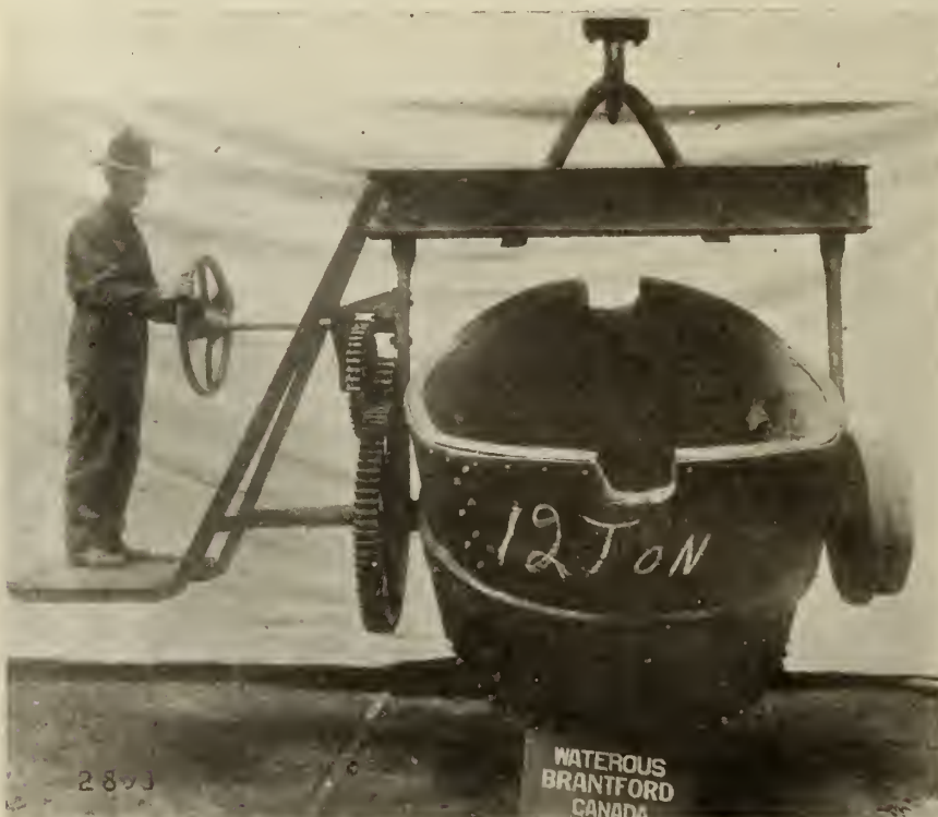
FIG. 3—A HANDY ATTACHMENT FOR LARGE CRANE LADLE.
