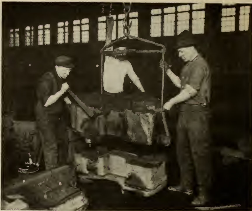
FIG. 2—MOLDING MOWER FRAME ON ROLL OVER TYPE STRIPPING PLATE MACHINE.
