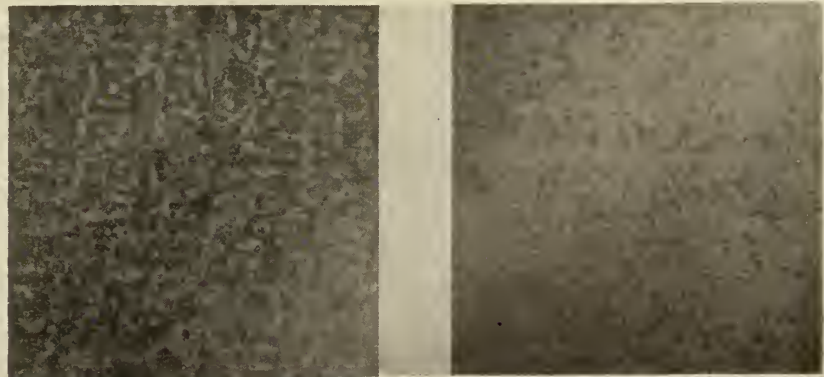
MICRO-PHOTOGRAPHS SHOWING POROSITY IN SAND CASTING DUE TO RELEASE OF ABSORBED GASES WHEN METAL FREEZES.
