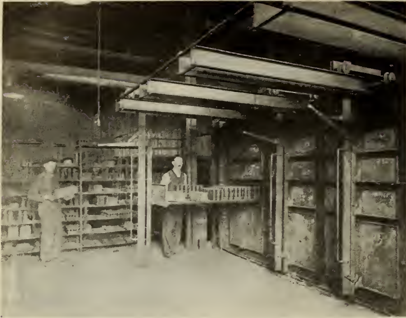
FIG. 2—OVEN AND RACK ROOM. FINISHED CORES ARE PLACED ON THE RACK AND TAKEN FROM THE OPPOSITE SIDE
