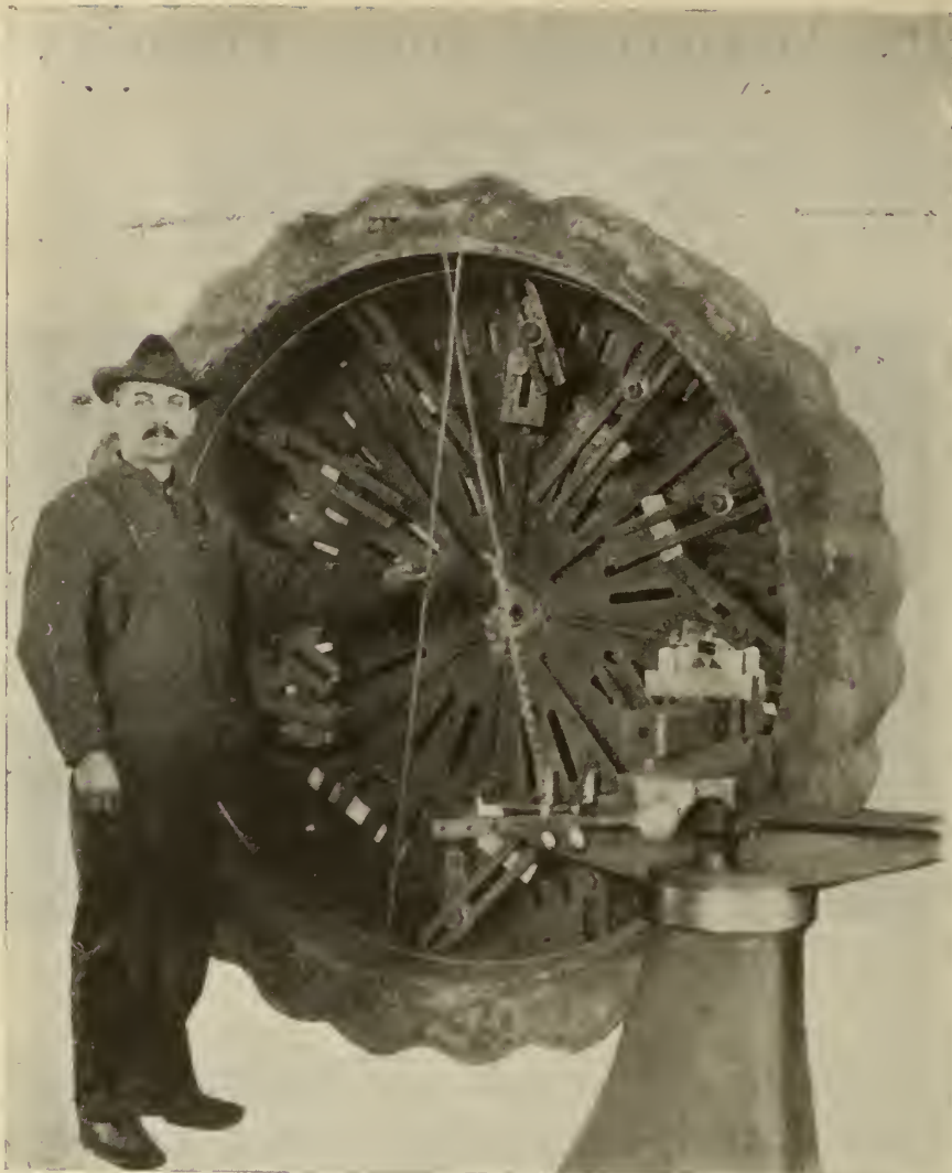
AN INTERESTING CHILLED CAST IRON ROLL TIRE, 79 IN. DIA., 20 IN. FACE, 7 IN. THICK, 7,625 LBS. CAST BY THE ASBESTOS FDRY. CO., INC., THETFORD MINES, QUE.
