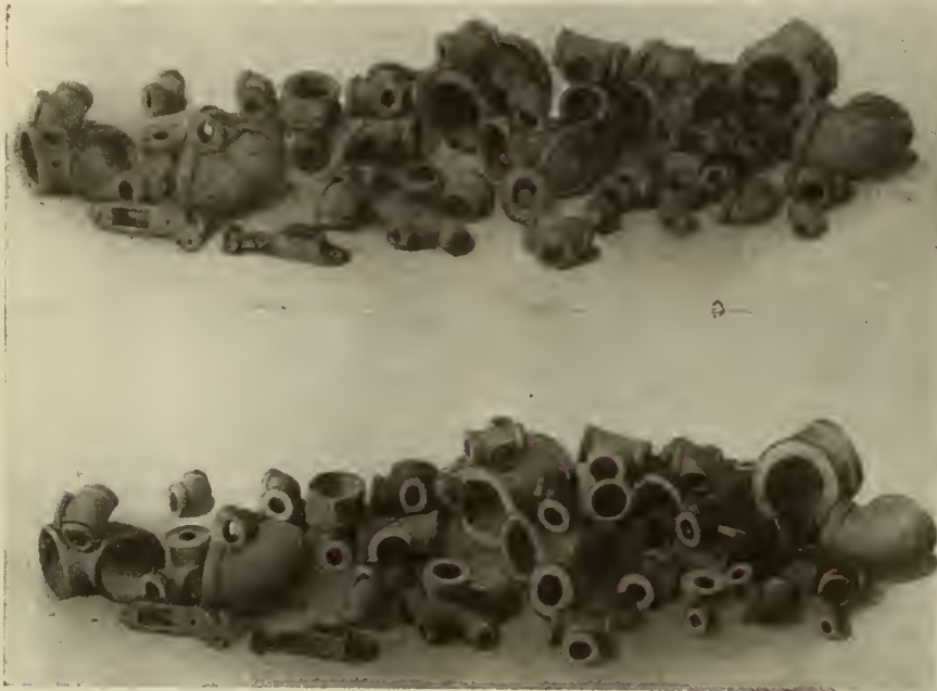
PLATE 16—FITTINGS CLEANED INSIDE AND OUTSIDE BY SUCTION TYPE OF SAND-BLAST
