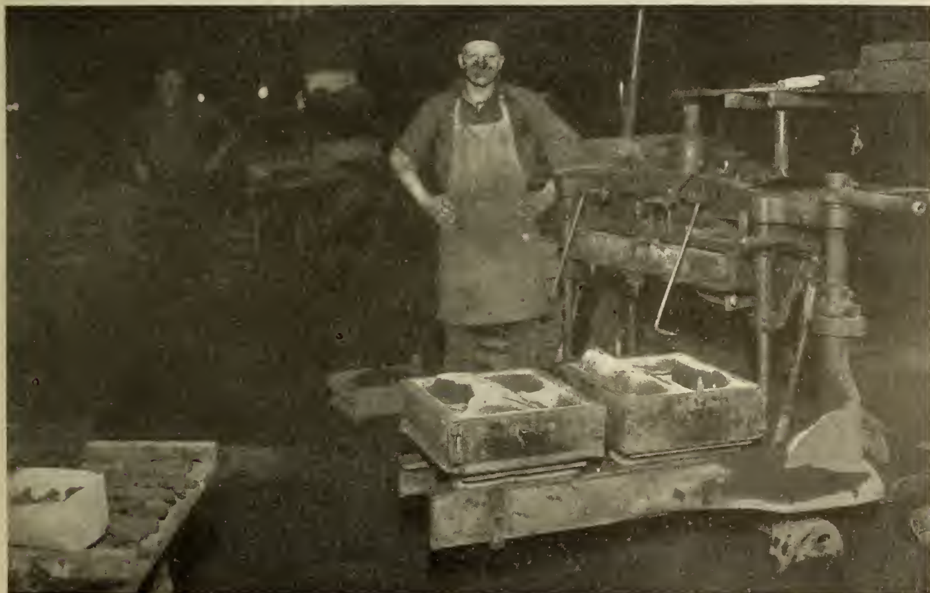
FIG. 1—COMBINATION JOLT RAMMER AND SQUEEZER MACHINE, RUN ENTIRELY BY PNEUMATIC POWER.
