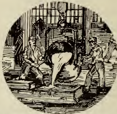
MODERN STEEL FOUNDRY PRACTICE HAS BEEN SO PERFECTED THAT TOP POURING CAN BE DONE SUCCESSFULLY ON MANY LINES OF WORK.
