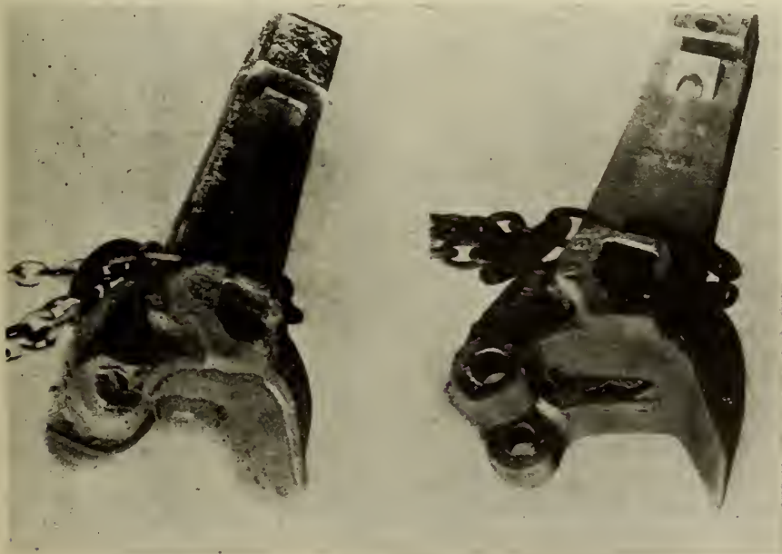
PLATE 11—STEEL CAR COUPLER CLEANED BY SAND BLAST
