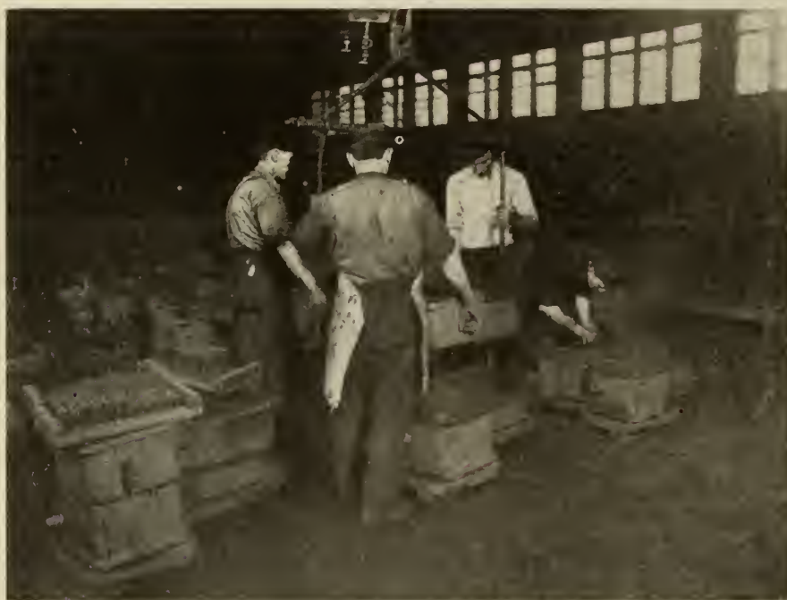
FIG. 3—CLOSING MOLD FOR MOWER FRAME. ALSO SETTING CORES IN ANOTHER
