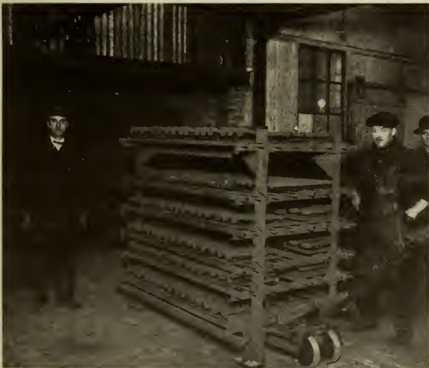
FIG. 5—ONE OF THE BATTERY OF CORE OVENS WITH CAR OF CORES READY TO BE SHOVED INTO OVEN. NOTE THE SIMPLICITY AND COMPLETENESS OF CAR.
