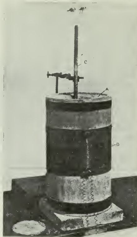
SELF-INDICATING ELECTRIC FURNACE FOR HARDENING STEEL.
