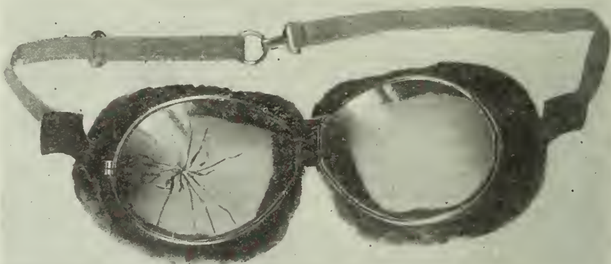
GOGGLES MAY HAVE THE OUTER GLASS CRACKED AND STILL THE LENS REMAINS INTACT WITH THIS PECULIAR METHOD OF LENS CONSTRUCTION.
