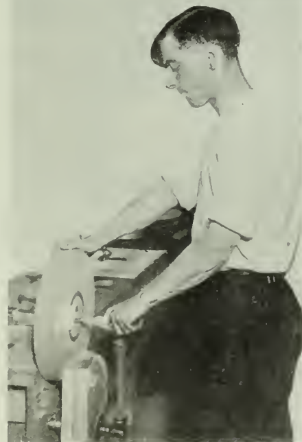
FIG. 2. REBUSHING GRINDING WHEELS.
