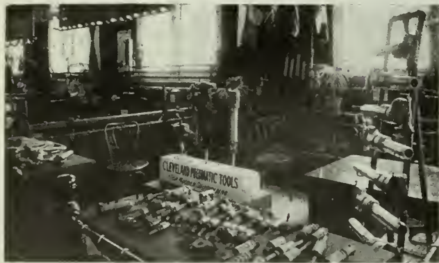
CLEVELAND PNEUMATIC TOOLS INCLUDED SPECIAL DESIGNS FOR WOOD SHIPBUILDING.
