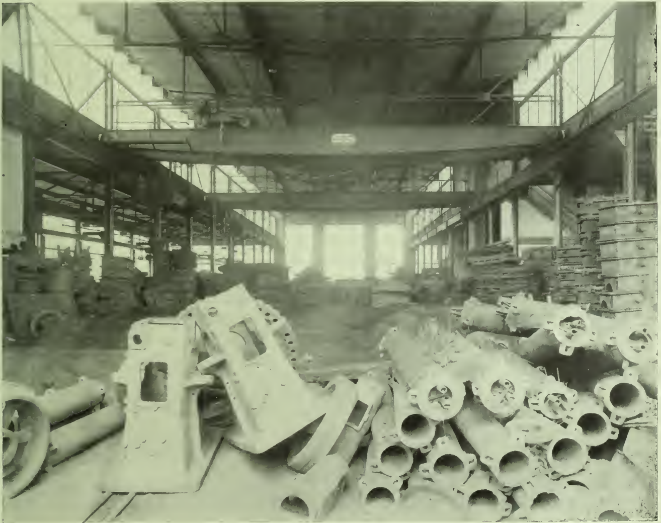
TWO 15-TON CRANES IN JAMES A. BRADY FOUNDRY, CHICAGO.
