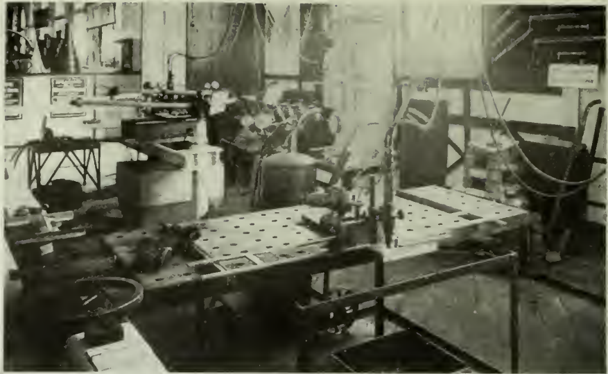
THE CARTER WELDING CO. SHOWED MECHANICAL APPARATUS FOR CUTTING AND SHAPING PLATES WITH OXY-ACETYLENE FLAME.
