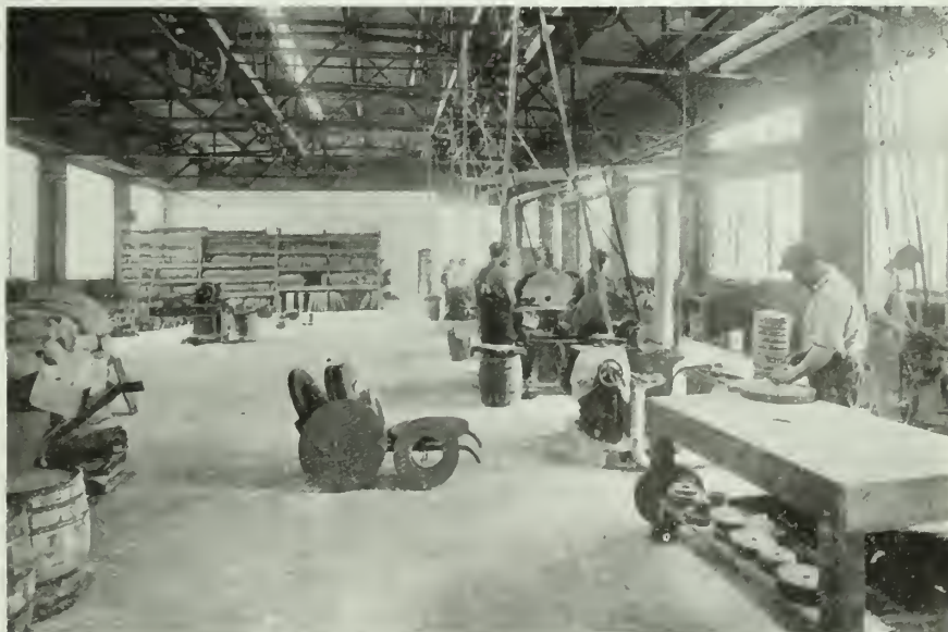
FINISHING DEPARTMENT, SHOWING TRUING WHEELS WITH DUST EXHAUSTING SYSTEM. WHEEL STORAGE IN BACKGROUND.
