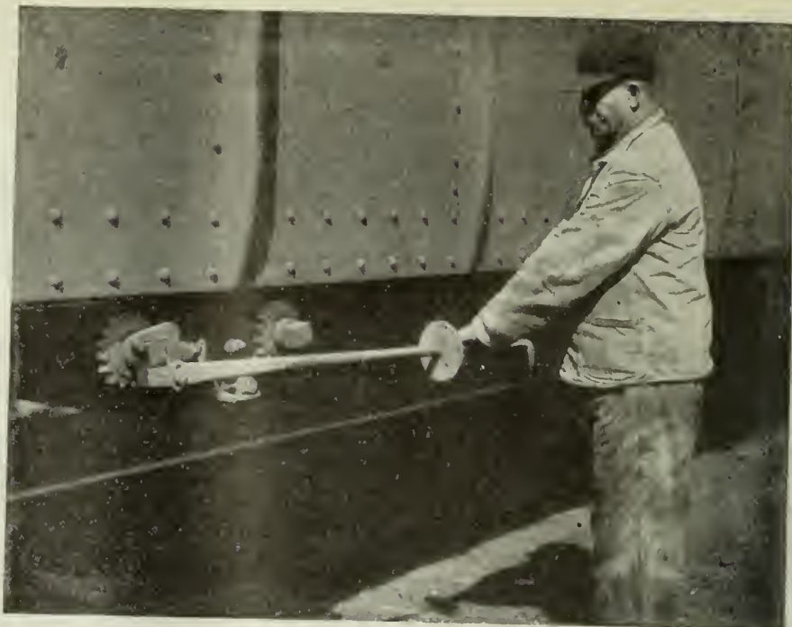
FIG. 23. TRESTLE LABORER USING SAFETY CAR WRENCH. WHEN THE SHAFT BEGINS TO REVOLVE, THE HINGED JAW RELEASES. DISC IS TO PREVENT MAN'S HAND STRIKING CAR, AND SHORT BEND ON END OF HANDLE PREVENTS USE OF PIPE EXTENSION.
