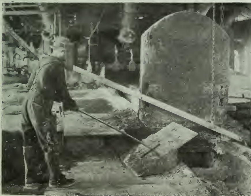
FIG. 15. SAFE METHOD OF OPERATING PUNCH-OUT GATE. Note the mask worn to protect man from splashes.
