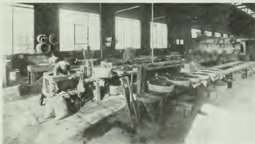
MIXING DEPARTMENT, SHOWING MIXING KETTLES AND GRINDING WHEEL MOULDS DRYING ON BENCHES. DRY-ROOM IN THE BACKGROUND.
