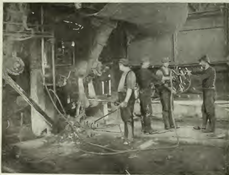
FIG. 14. SAFE METHOD OF DRILLING A TAPPING HOLE.
