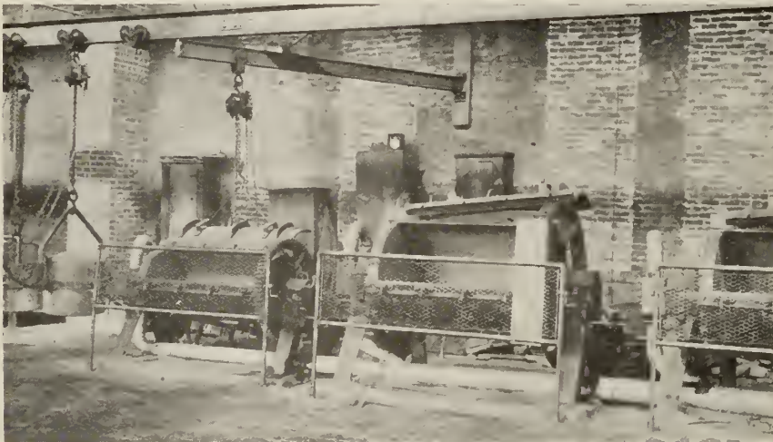
GUARDS MADE OF WOVEN WIRE AND PIPE FOR PROTECTING TUMBLING BARRELS.
