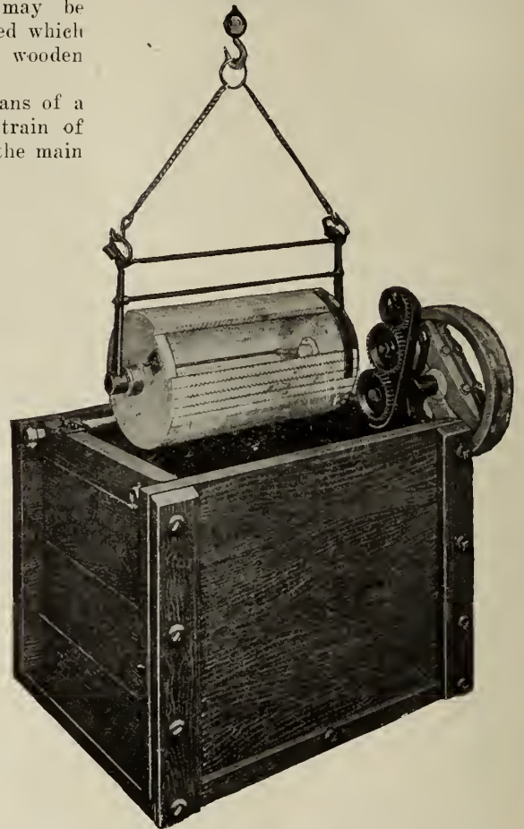
FIG. 2. BARREL RAISED CLEAR OF TANK FOR REMOVING WORK, GIVING ACCESS TO LIQUID.
