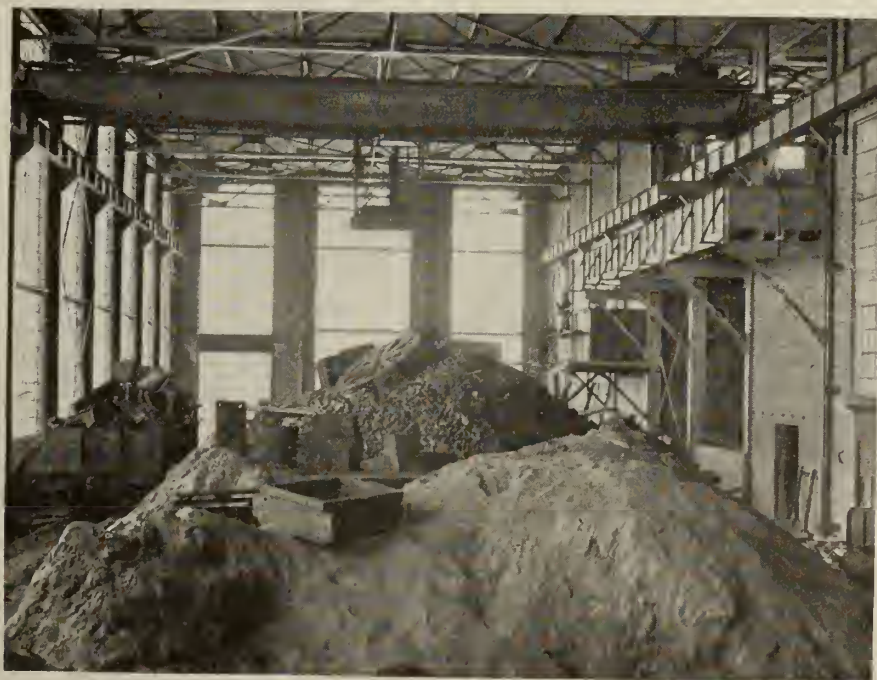
NEW GREY IRON FOUNDRY, STORAGE BAY FOR RAW MATERIALS SHOWING CHARGING FLOOR UNDER RIGHT-HAND END OF TRAVELING CRANE.
