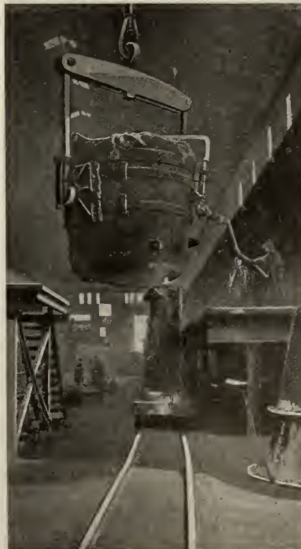
POURING 3-TON INGOTS, SYDNEY MINES.
