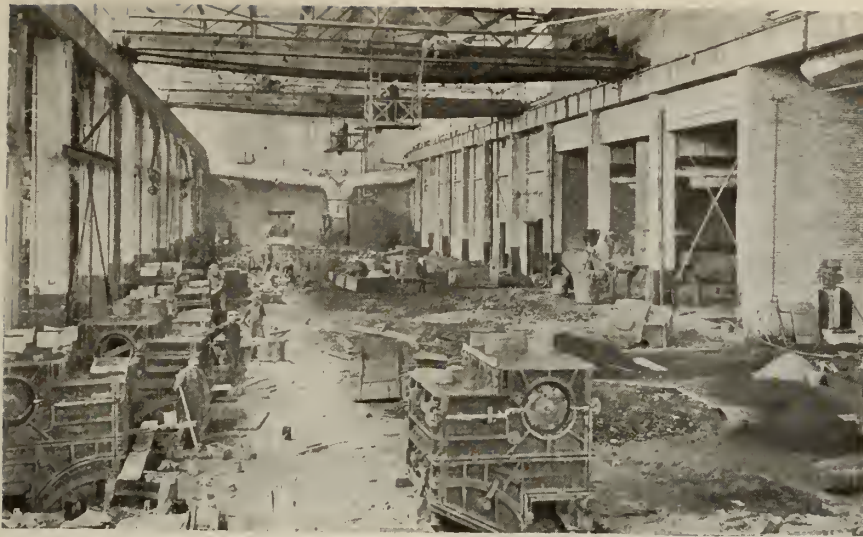
NEW GREY IRON FOUNDRY, NORTH END OF MOLDING FLOOR FOR HEAVY CASTINGS.
