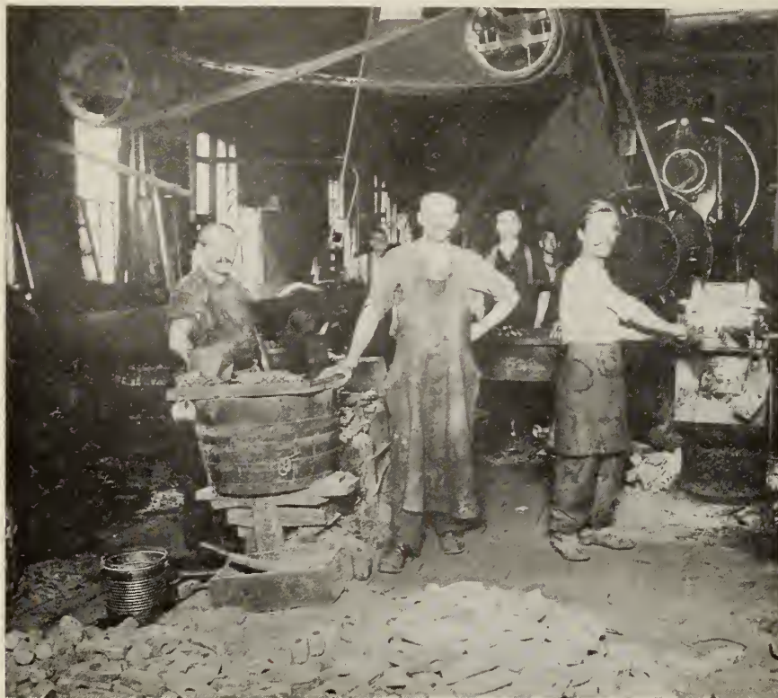
MAKING SLEDGE HAMMERS IN THE FORGE SHOP.
