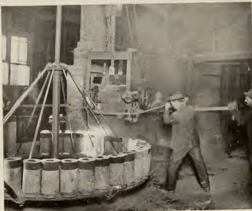
FIG. 3. CASTING 4.5 SHELL BILLETS IN INGOT MOLDS.
