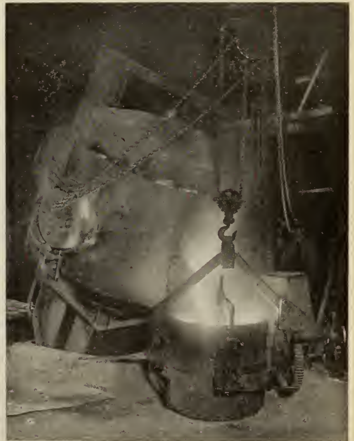
FIG. 2. TAPPING THE FURNACE INTO LADLE.
