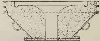
FIG. 5. CONICAL SECTION OF FLASK AFTER DRAWING PATTERN.
