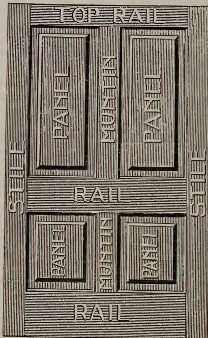
DOOR, SHOWING CUTTINGS.
