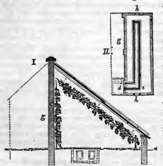
a simple plan of a vinery of this kind. In this the surface of the ground is shown at  $\alpha$ , below which, the foundation walls are sunk three feet. Above the surface the front wall b, rises two feet, the back wall c, twelve feet, and the width of the house is fourteen feet. On these walls are placed the rafters, from three to four feet distant. with the sashes in
