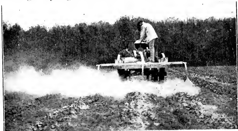
FIG. 229.—Three-row duster operated by gas engine; used on strawberries to combat weevils. (New Jersey Station.)
