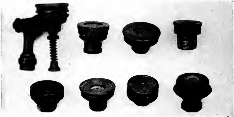
FIG. 227.—Several types of spray nozzles. All modern nozzles have a large disk in which the liquid is given a rotary motion before exit from the orifice. (New Jersey Station.)
