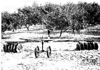
FIG. 234.—A common disk harrow may be attached to the ends of an extension bar to cultivate under orchard trees. (New Jersey Station.)
