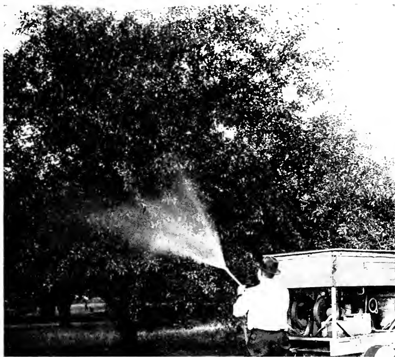
FIG. 225.—With a gasoline or oil engine a high pressure may be easily maintained. This makes a fine mist. (Michigan Station.)
