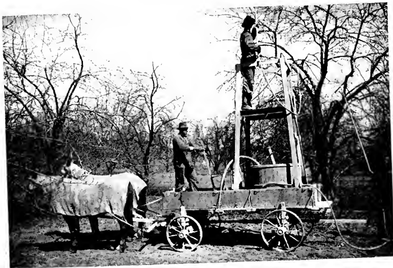
FIG. 224.—A double-acting hand pump and tank arranged to spray through two leads of hose from a farm wagon. From the tower platform the tops of orchard trees may be sprayed. (Indiana Station.)
