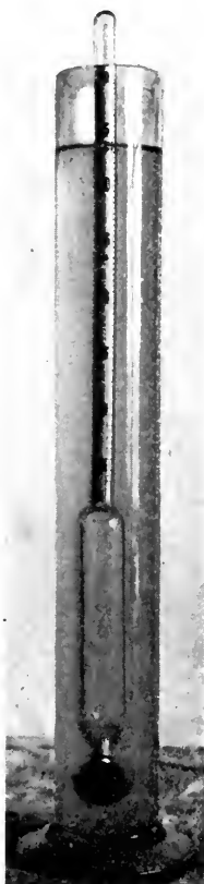
FIG. 216.—Hydrometer and cylinder for use in testing the density of lime-sulfur and other spray materials. It is scaled by the Baumé standard. See table in appendix. (Indiana Station.)
