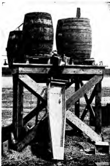
FIG. 214.—An elevated platform for mixing Bordeaux and other spray materials. Two barrels may be used for stock solutions and others for the dilute mixture. The extension trough aids in filling the spray tank which is hauled near the platform. (Indiana Station.)
