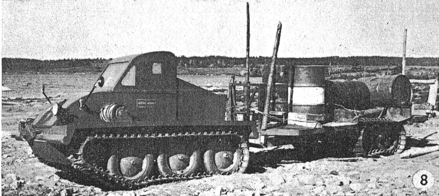
Figure 7—Burning in a lowbush blueberry field with an oil burner. This type of machine works well on smooth land.
