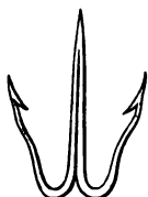
FIG. 62. DOUBLE BRAZED HOOK.
